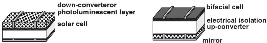
Figure 1.10: (a) solar cell with downconverter added to the front side; (b) solar cell with upconverter on the rear side.
