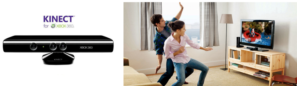
Figure 1.5 – Microsoft Kinect sensor (left image) and a sample image presenting a human-computer interaction (right image).
