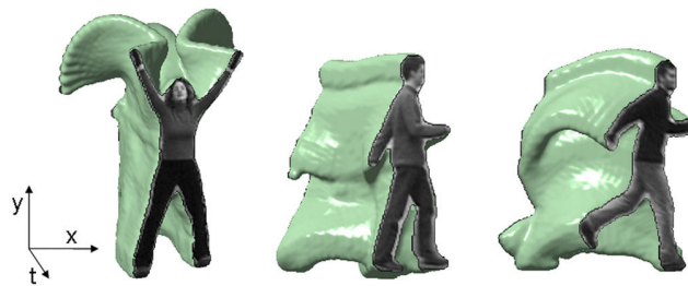
Figure 2.7 – Blank et al. [Blank 2005]: Sample spatio-temporal volumes constructed by stacking silhouettes over a given sequence.
