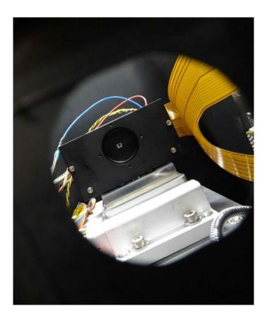
Figure III.13: **Baffle v2.** The picture is taken in front of the chip, just behind the outer vane inside the vacuum chamber. The small square inside the bright area is the sensitive area of the chip. The black square around the bright area next to the chip is the inner vane.
