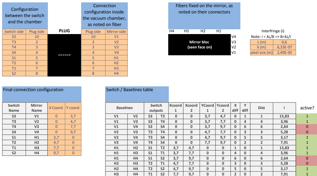
Figure E.6: Metrology configuration spreadsheet. It summarize all the practical information needed about the current metrology configuration: how the connectors/fibers are paired between the switch and the vacuum plug, after the vacuum plug inside the vacuum chamber, what are the final baselines interfringe distances and what are the corresponding switch commands.
