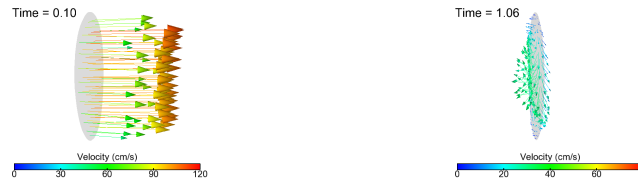
Figure 5.6: Velocity fields during maximal forward flow (left, t=0.10s ) and reverse flow (right, t=1.06s ) at the LPA interface with the 3D-3D-0D coupling approach.
