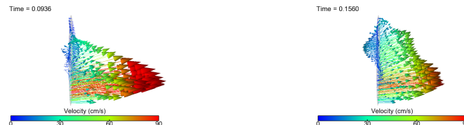
Figure 5.12: RPA velocity fields during peak flow (left) and decelerative flow (right) with the 3D-3D-0D method.
