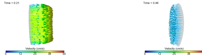
Figure 5.18: Velocity fields at two different time points ( t=0.21s (maximal forward flow at inlet) on the left side and t=0.46s (maximal reverse flow at outlet) on the right side) by using 3D-3D-0D model.
