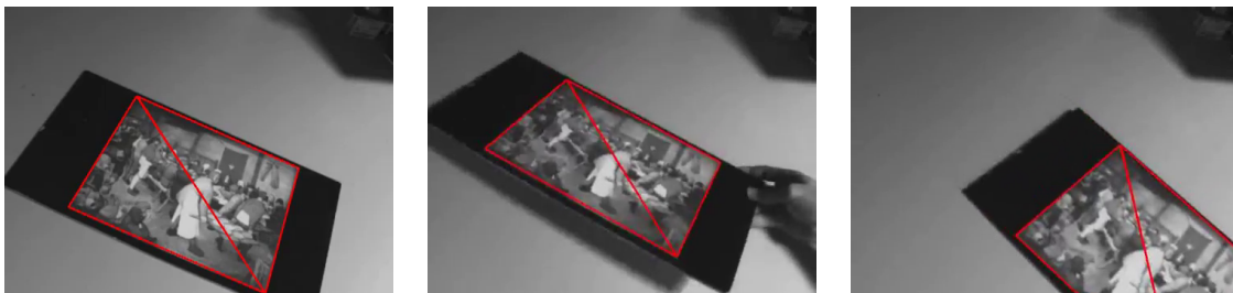
Figure 2.3: Example of visual tracking using the SSD as registration method [Baker and Matthews, 2004] using the ViSP library [Marchand et al., 2005].
