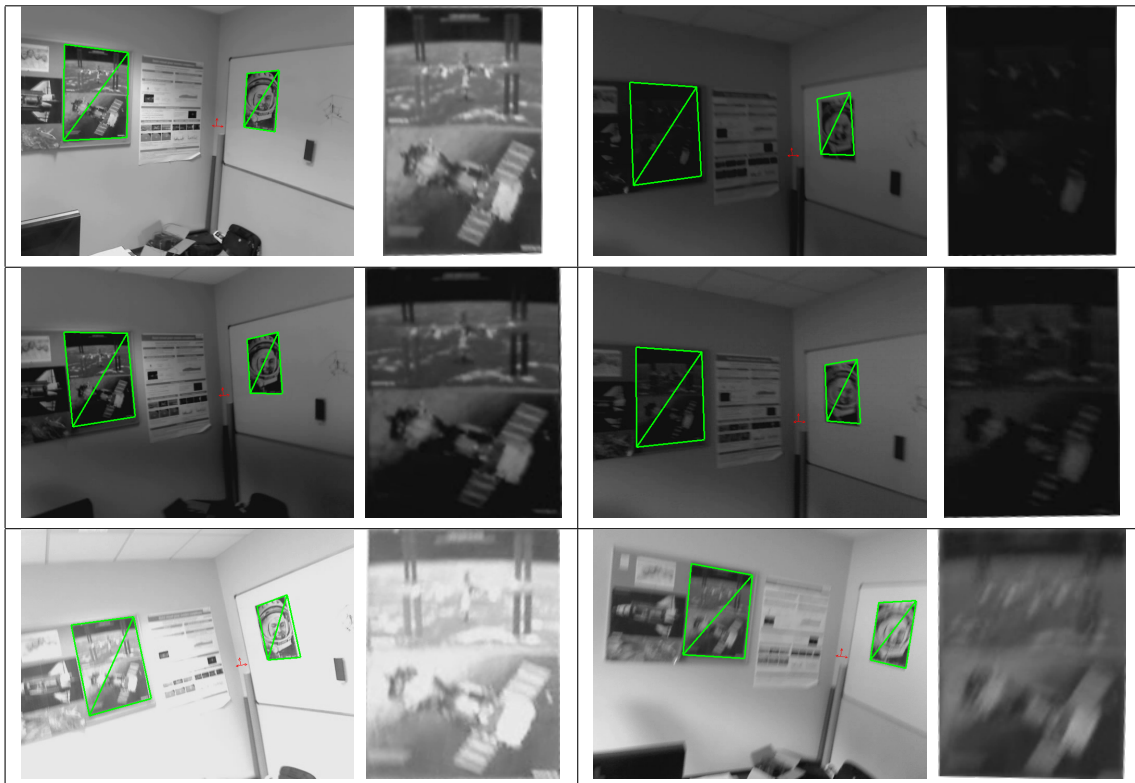
Figure 3.8: On the left of each pair is the tracking result of our MI algorithm and on the right what is actually seen in the image at the place of the left face. Let us add that the patch is very blurred on several occasions but the tracking is still successful.
