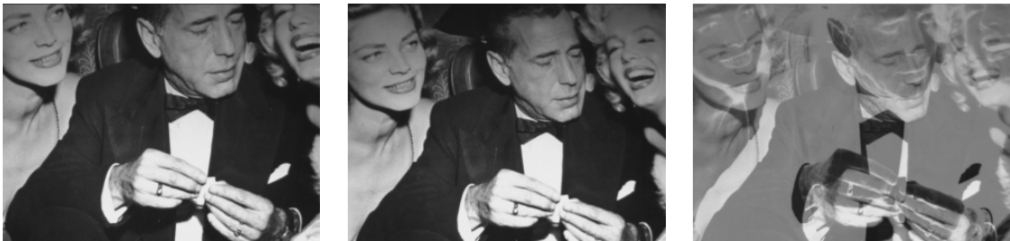
Figure 6.3: From left to right: image seen at desired and start position and corresponding image error. Pixel values on the image error are shifted by an offset of 128 grey levels in order to increase readability.
