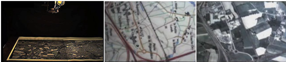
Figure 5.8: Visual navigation using the MI. From left to right: Servoing robot setup, current desired image along the visual path and current image perceived by the camera mounted on the robot.
