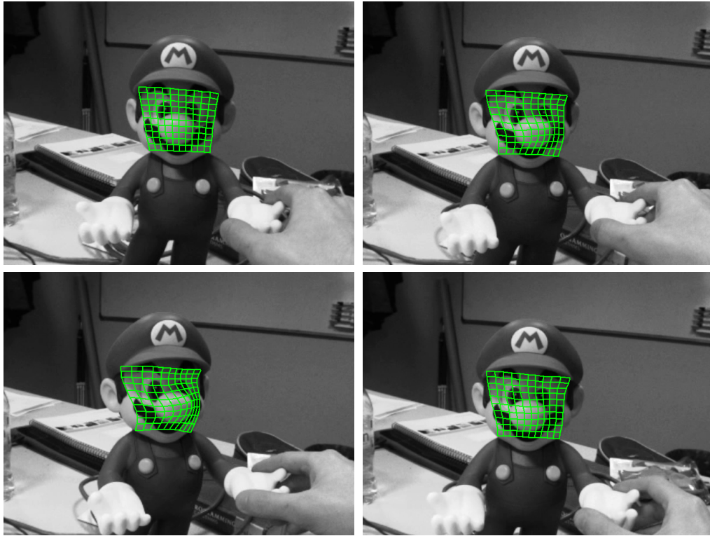
Figure 4.10: Results of the tracking algorithm on a three dimensional object. There again the tracking is successful even when a part of the object is occluding another one.
