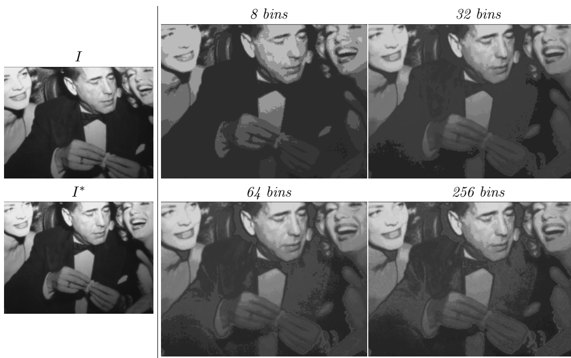
Figure 6.1: Influence of the number of bins on the predicted image. On the left, with 8 bins the image is flattened and has lost a lot of high frequencies. 256 bins introduces more noise when the difference between I and I^* increases than 64. The frame on the borders represent the area in the image which is not included in the computation.
