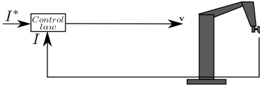
Figure 5.6: Classical dense visual servoing loop. The current image is directly compared to the image recorded at the desired position in order to compute the velocity vector \mathbf{v} .
