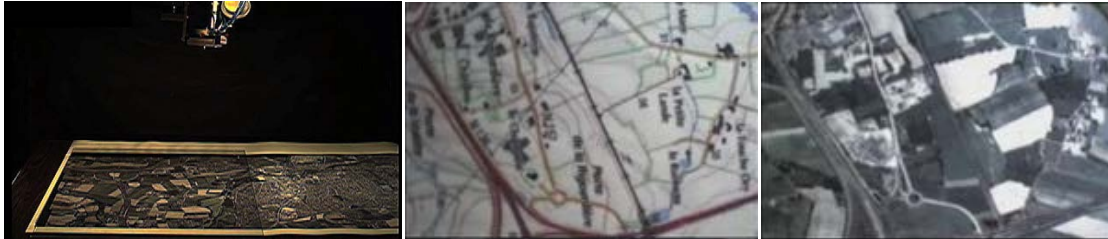
Figure 5.8: Visual navigation using the MI. From left to right: Servoing robot setup, current desired image along the visual path and current image perceived by the camera mounted on the robot.
