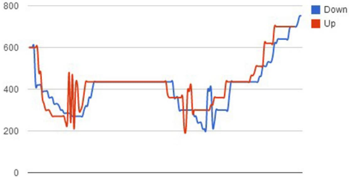
Figure 3.3: Initial handmade timetable : graph representing the headways in seconds in function of the metro departure times. The red line represents the metros running upstream and the blue line the metros running downstream.
