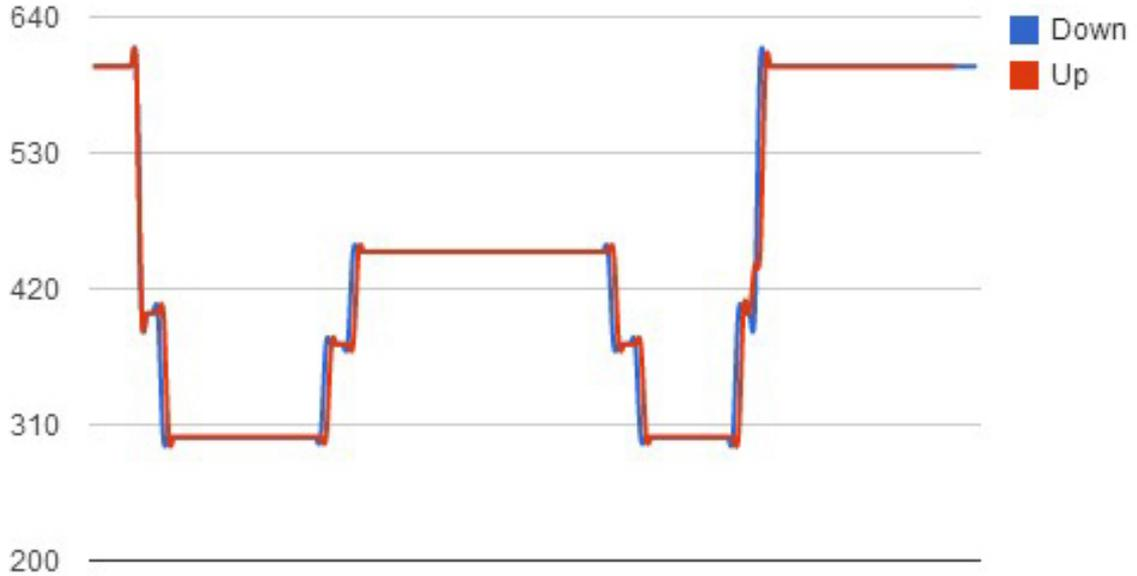
Figure 3.4: Compiled timetable following the given headway pattern : graph representing the headways in seconds in function of the metro departure times. The red line represents the metros running upstream and the blue line the metros running downstream.
