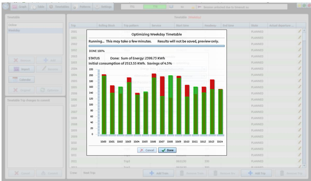
Figure 6.1: Screenshot of the ATS optimization module of the General Electric Transportation signalling system.
