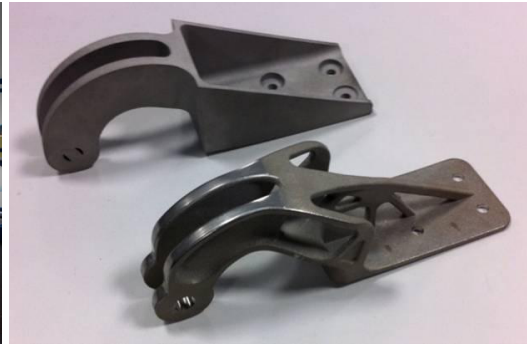
(b) A conventional hinge is seen in the background and a 3D-printed metal hinge is seen in the foreground - EADS.
