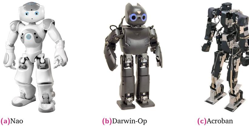
Fig. 6.1.: None of the existing platforms in 2012 was suitable for exploring the role of morphology. Nao was impossible to modify. Darwin Op and Acroban used aluminium parts that are really difficult and expensive to produce.
