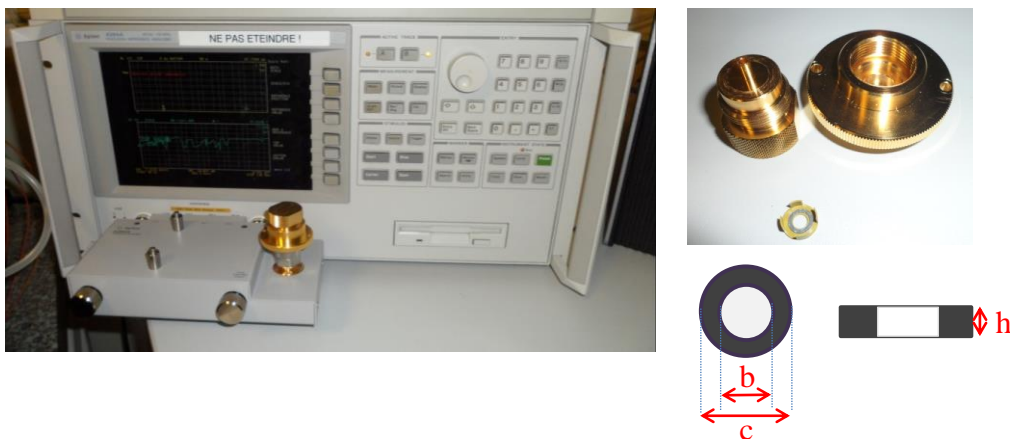
Figure 3-4: Complex permeability measurement set-up; b and c : respectively internal and external diameter of the toroid; h : thickness of the toroid
