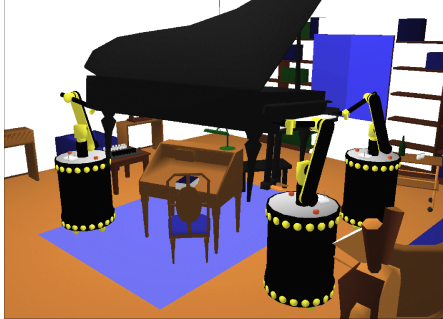
Fig. 1. A “closed-chain” version of the piano mover’s problem. The piano is moved by three cooperating mobile manipulators, creating multiple closed kinematic chains.
