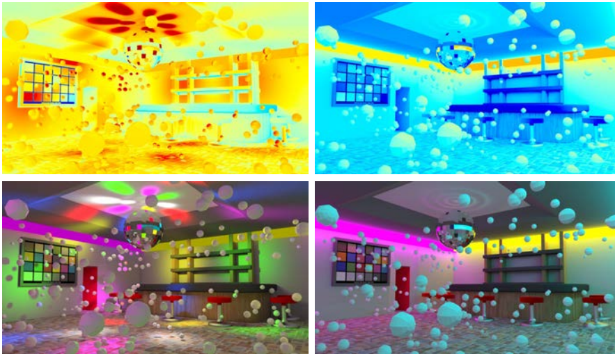
Figure 3.6: Example of a temporal contrast incoherency when a change of illumination occurs. False color luminance (top row) and tone mapped result using [Reinhard et al., 2002] operator (bottom row). Both frames appear at the same level of brightness although the false color representations indicate different levels.
