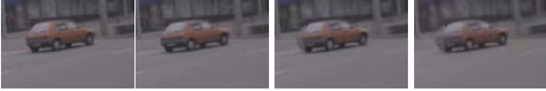
Figure 6.5: Zoom on the decoded frame 2 of the Tunnel sequence (TMO = [Ramsey et al., 2004]) at bit-rates 1000, 500, 250 and 125 kbps (from left to right). Artifacts around the red car appear for bit-rates 250 and 125 kbps. Corresponding PSNR with the original frame 1000 kbps = 40.82 dB, 500 kbps = 40.20 dB, 250 kbps = 38.85 dB and 125 kbps = 37.71 dB.
