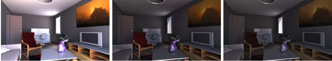
Figure 2.12: Comparison of Edge-Aware TMOs using only one detail layer. From left to right: bilateral filter [Durand and Dorsey, 2002], weighted least square filter [Farbman et al., 2008] and recursive filter [Gastal and Oliveira, 2011].
