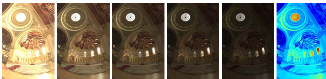
Figure 2.5: 1 st to 5 th images: different exposures of the same scene, two successive images are separated by 4 f-stops. Rightmost image: false color representation of the generated HDR image.
