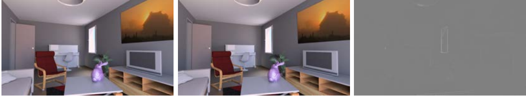
Figure 2.10: Comparison of the global and local version of [Reinhard et al., 2002] operator. From left to right: global, local and difference in luma.
