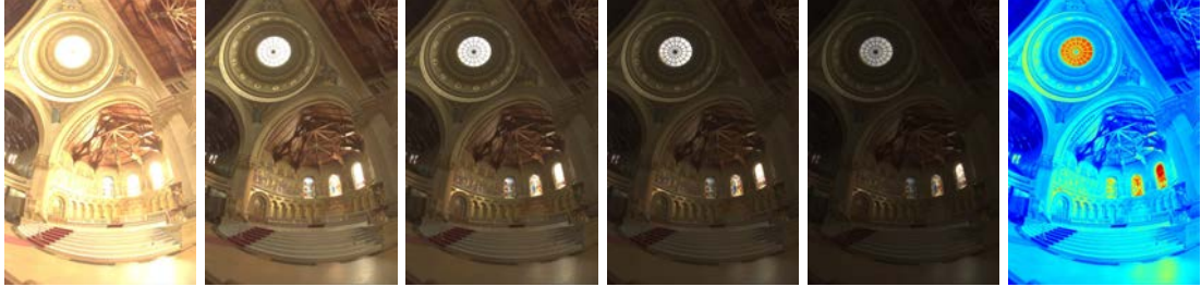
Figure 2.5: 1 st to 5 th images: different exposures of the same scene, two successive images are separated by 4 f-stops. Rightmost image: false color representation of the generated HDR image.
