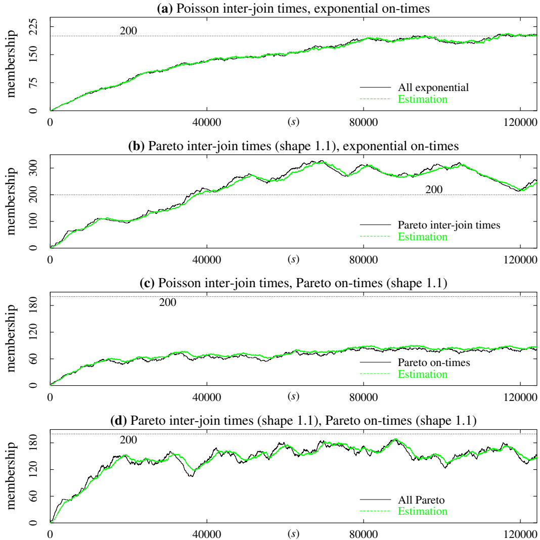
Figure 2.4: Estimation of the multicast membership over time ( p = 0.01, S = 1s ): the heavy load case \lambda T = 1/185.9s^{-1}, \mu = 1/37180s^{-1}
