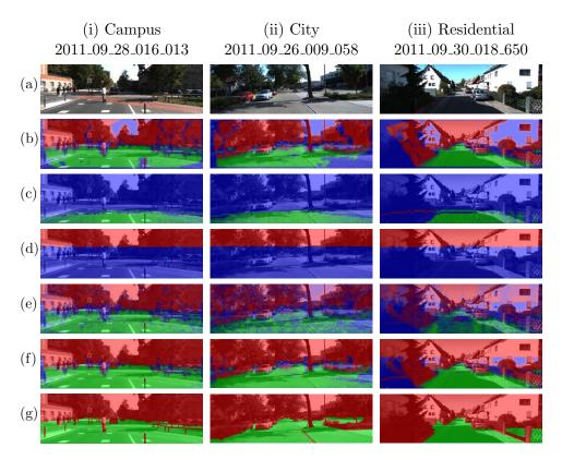
Figure 5.9: Classification from the ground detection modules. The RGB colors represent the mass assigned to  $\{ground\}$ ,  $\{ground\}$  and  $\Omega_G$ , respectively. (a) Raw images. (b) Stereo-based module. (c) LiDAR module. (d) Pixel-based module. (e) Temporal propagation of the combined mass function from the previous frame. (f) Combined mass functions. (g) Ground truth images.
