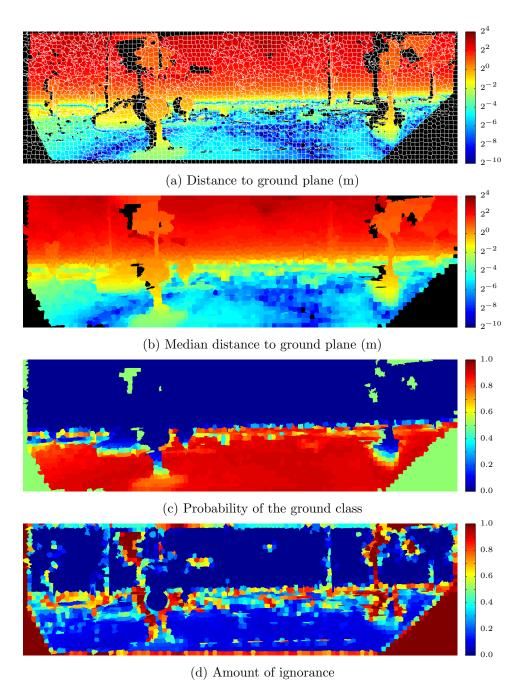
Figure 5.5: Stereo-based ground classification. (a) Distance to the ground plane for each pixel. (b) Median distance of segments to the ground plane. (c) Probability of the ground class  $P_d^{\Omega_{\rm G}}$ . (d) Amount of ignorance  $m_{\underline{d},\overline{d}}^{\Omega_{\rm G}}(\Omega_{\rm G})$ .
