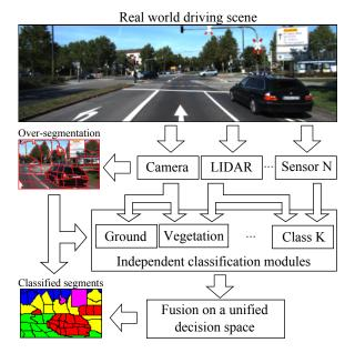
Figure 5.1: Overview of the fusion framework. N sensors, including a camera, observe the scene and provide data to K independent modules. The classification outputs are then fused in a unified decision space built from an over-segmented image.
