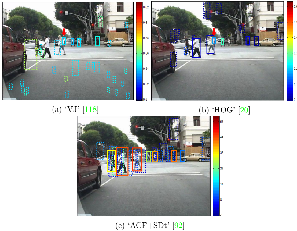
Figure 4.2: Pedestrian detection results from three algorithms. The colour of the bounding boxes represents the score. Solid boxes are true positives and dotted boxes are false positives. The red arrow points to a pedestrian detected by both 'VJ' and 'HOG' but not 'ACF+SDt'.
