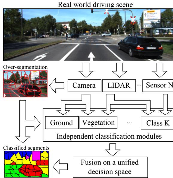
Figure 5.1: Overview of the fusion framework.  $N$  sensors, including a camera, observe the scene and provide data to  $K$  independent modules. The classification outputs are then fused in a unified decision space built from an over-segmented image.
