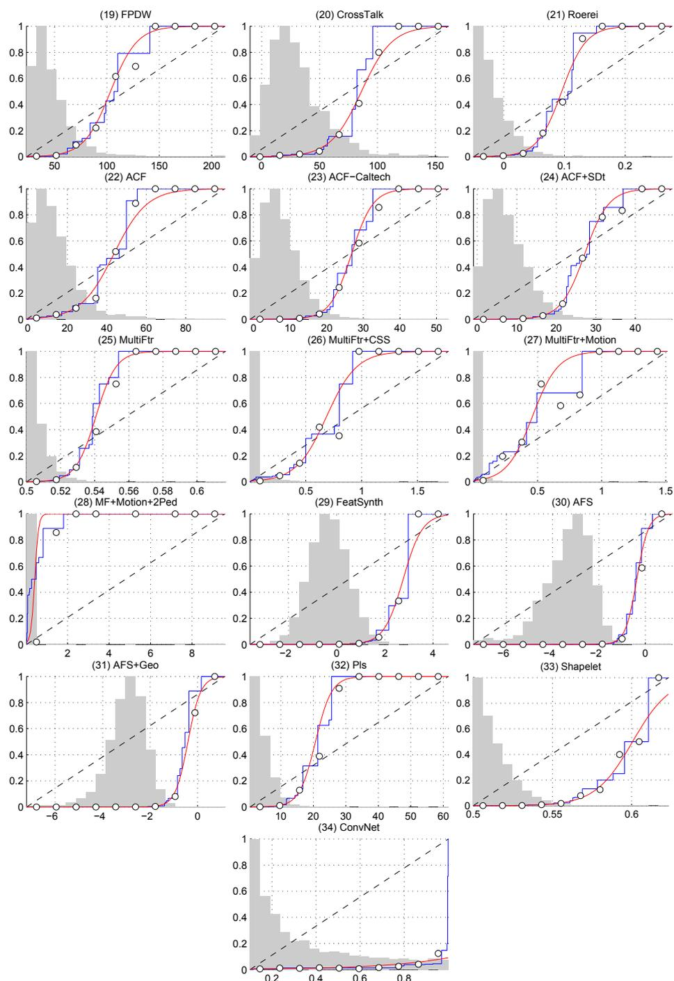
Figure 4.5: Calibration of pedestrian detectors. The  $x$ -axis corresponds to the raw scores returned by the detectors and the  $y$ -axis corresponds to the calibrated posterior probability. The white dots correspond to binning using ten equally spaced bins. Isotonic and logistic regression based calibration are represented, respectively, by the blue and red curves. The gray bars represent the empirical normalized distribution of the scores.
