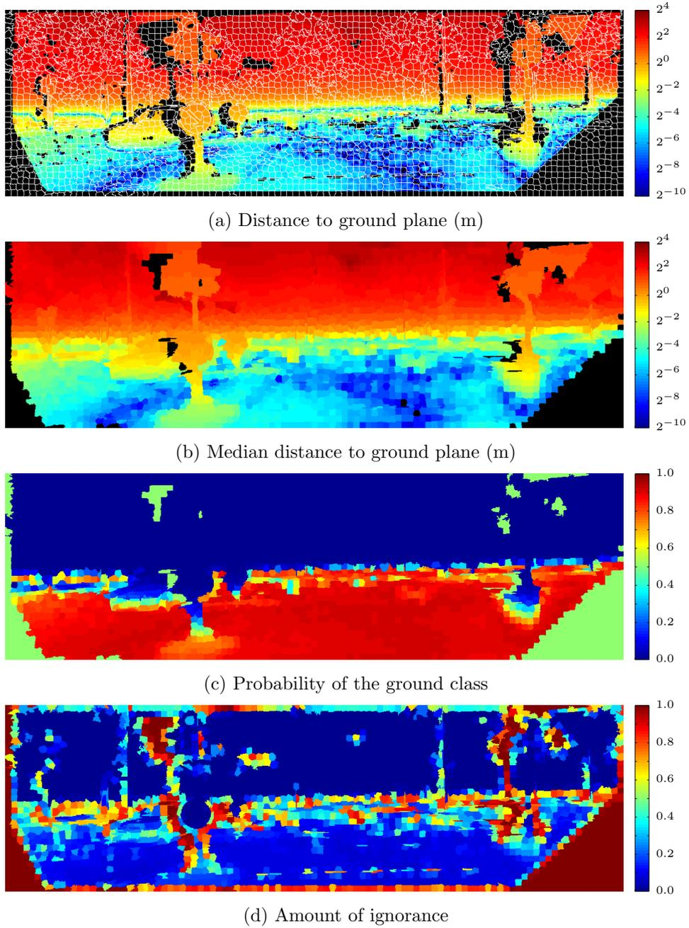
Figure 5.5: Stereo-based ground classification. (a) Distance to the ground plane for each pixel. (b) Median distance of segments to the ground plane. (c) Probability of the ground class  $P_d^{\Omega_G}$ . (d) Amount of ignorance  $m_{d,d}^{\Omega_G}(\Omega_G)$ .
