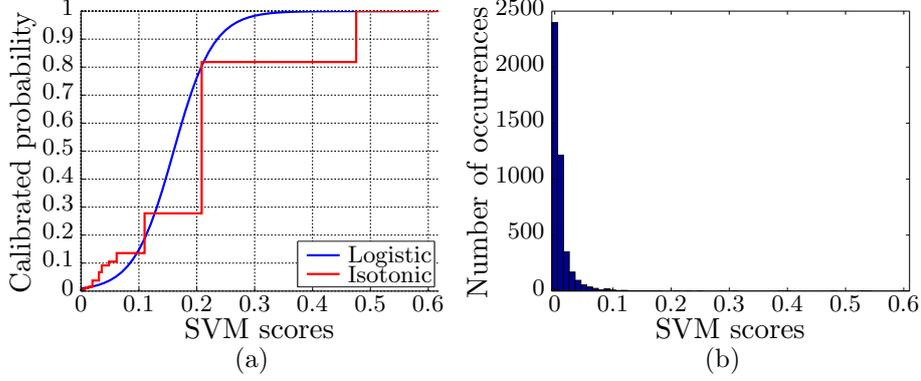
Figure 4.3: (a) Logistic and isotonic calibration of the scores from the ‘HOG’ pedestrian detector. (b) Histogram of the scores.
