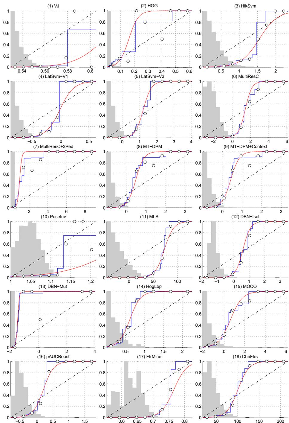
Figure 4.4: Calibration of pedestrian detectors. The  $x$ -axis corresponds to the raw scores returned by the detectors and the  $y$ -axis corresponds to the calibrated posterior probability. The white dots correspond to binning using ten equally spaced bins. Isotonic and logistic regression based calibration are represented, respectively, by the blue and red curves. The gray bars represent the empirical normalized distribution of the scores.
