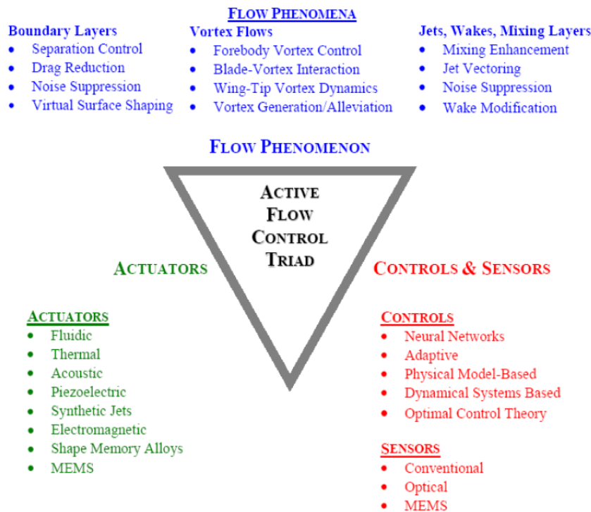
Figure 1.8: The feedback flow control triad. (Courtesy D. E. Parekh, Georgia Tech Research Institute)
