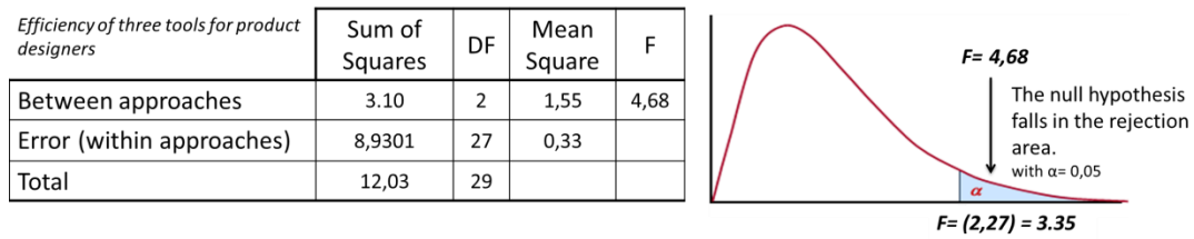
Figure 4-28: Results of ANOVA test for comparison of the efficiency of three approaches among product designers
