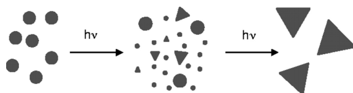
Figure I.19 - Conversion of silver nanospheres into nanoprisms. [Jin01]
