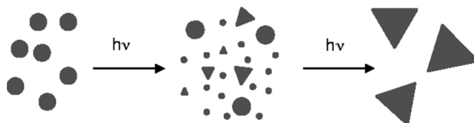
Figure I.19 - Conversion of silver nanospheres into nanoprisms. [Jin01]
