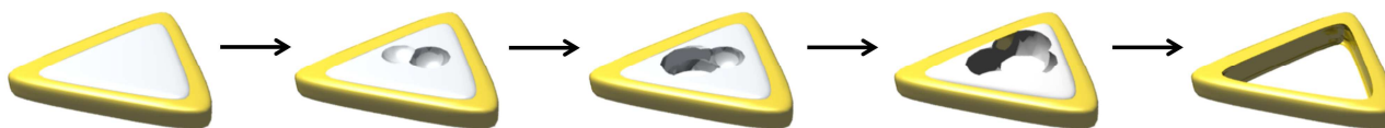
Figure A.11 - Formation of a triangular gold nanoring from a silver nanoprism.
