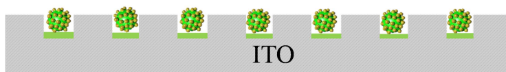
Figure A.25- Schematic illustration of a substrate presenting a network of lithographed holes in which only one nanocluster could be deposited.
