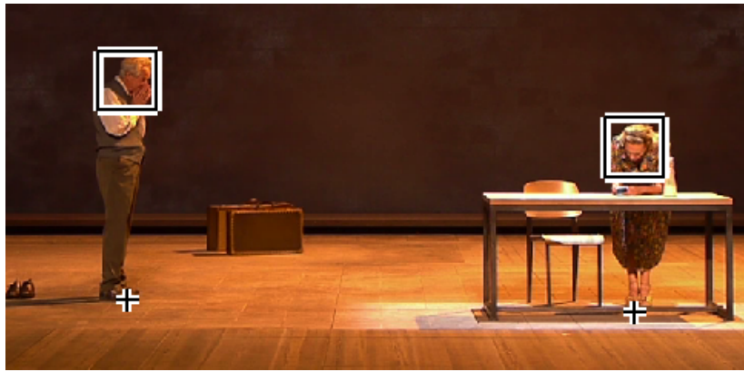
Figure 7.2: Input to the system are the upper body bounding boxes for each actor (shown with squares) and the points where the actors touch the stage floor (shown with cross markers).
