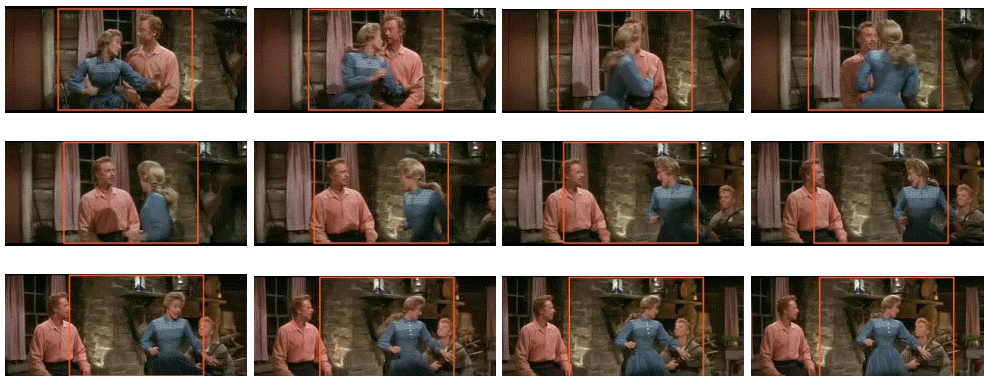
Figure 3.1: Illustration of pan and scan. The red rectangle shows the pan and scan version of the original frame in wide-screen format. Images reproduced from http://www.videohelp.com .
