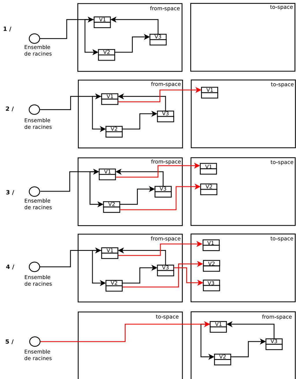
Figure 1.3 – Algorithme *Stop&Copy*
