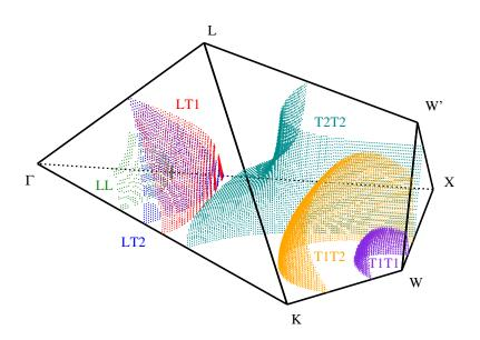
Figure 3.12: 3D pictures of the two-phonon final states of the X-zone-edge LA-phonon decay through Umklapp processes in SiSn. The channels classification is as follows: LL: LA+LA, LT1: LA+TA1, LT2: LA+TA2, T1T1: TA1+TA1, T2T2: TA2+TA2, T1T2: TA1+TA2
