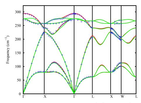
Figure 2.4: Phonon dispersion relation of bulk GaAs with (red) and without (green) taking into account the coupling between electric field at atomic vibration. Experimental data (blue points) are reproduced from [114].
