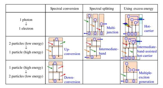
Figure 1.2: Types of solar cells to exceed the Schockley-Queisser limit. Reproduced from [8]
