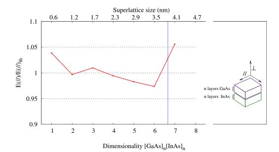
Figure 4.5: Relative electric field induced by the in-plane all-couples-in-phase vibration mode (number (6) in figure 4.7) upon dimensionality. The reference value  $E_{th}$  is the exact average of bulk GaAs and InAs (see text). The blue dashed line indicates the (rough) separation between superlattices and quantum wells from a phonon point of view (4.1).
