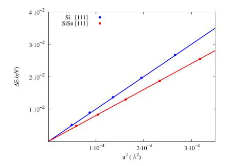
Figure G.1: Energy distortion  $\Delta E$  as a function of the displacement u along the [111] direction for Si and SiSn.
