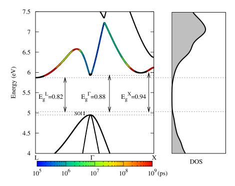
Figure 3.9: (Left)  $G_0W_0$  corrected DFT calculated SiSn electronic band structure. The color of the first conduction band illustrates the corresponding LO phonon lifetime at 300 K via intra-valley scattering (see text). The slope remains black if no phonon fulfilling equations (2.14) and (2.15) is found. (Right) Electronic density of states.
