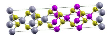
Figure 4.1: Crystal unit cell of  $[InGaAs]_4$ . In, Ga and As atoms are coloured in grey, pink and yellow rescrectively.
