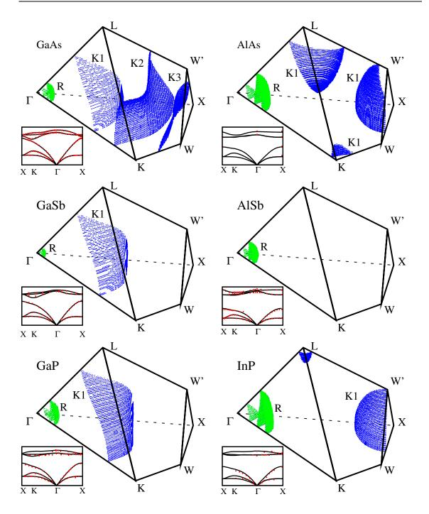
Figure 2.6: Two-phonon final states in the zone-centre approximation for III-V semiconductors. The blue surfaces are Klemens states (K1, K2 and K3 for first, second and third Klemens states), the green ones are Ridley states (R). The insets show the accordance between computed dispersion relation and experimental data on high symmetry lines([114, 107, 128, 129, 130, 131, 132, 133, 134]).
