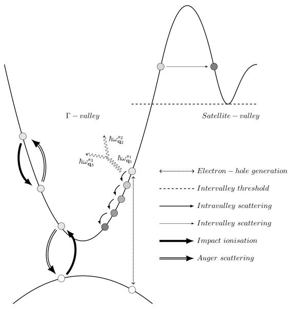
Figure 1.3: Hot electrons cooling processes.
