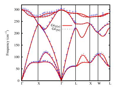
Figure E.1: Transferability of the force constant from Si to Ge. The Ge band structure has been calculated using the force constant of Ge (red solid line) and Si (black dashed line), and is compared to experimental values reproduced from [186] (blue crosses).
