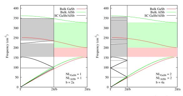
Figure 2.3: Band folding and mini-gaps formation in one-dimensional  $(GaSb)_{NL} - (AlSb)_{NL}$  superlattice, NL being the number of layers of each compound. The lattice parameters of GaSb and AlSb are considered to be identical, and equal to a, so that the superlattice one is b = 2aNL. The shaded areas highlight the forbidden energy range for bulk GaSb (red), bulk AlSb (green), and the superlattice (grey).
