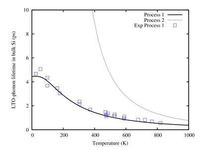
Figure 3.6: LO-phonon decay (process 1) and creation (process 2) in a three-phonon interaction in Silicon. Experimental data are reproduced from [125].
