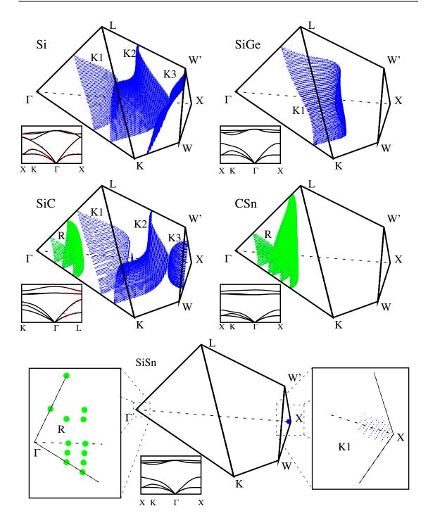
Figure 2.7: Two-phonon final states in the zone-centre approximation for group IV semiconductors. The blue surfaces are Klemens states (K1, K2 and K3 for first, second and third Klemens states), the green ones are Ridley states (R). The insets show the accordance between computed dispersion relation and experimental data whenever they exit ([99, 135]).
