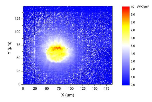
Figure 1.8: Local measurement of the thermalisation rate deduced from an absorbed power map based on integrated PL map and the corresponding local temperature map of emission under 22000 suns. Reproduced from [22]
