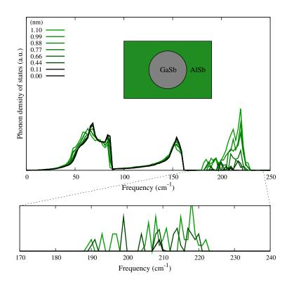
Figure 2.14: Phonon density of states of different sized GaSb quantum dot embedded in an AlSb matrix. The legend indicates the dot radius.
