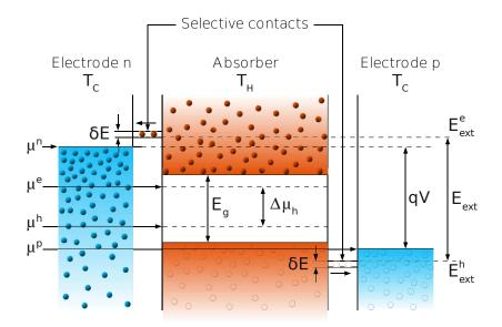
Figure 1.4: Principle of a hot-carrier solar cell. Reproduced from [7]
