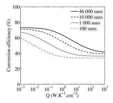
Figure 1.5: Efficiency of a hot-carrier solar cell with a 0.7 eV band gap absorber (as in GaSb) and perfectly selective contacts as a function of the thermalisation coefficient  $\mathbb{Q}$  for different concentrations of the incident radiation. Reproduced from [7]
