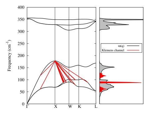
Figure 3.11: 2D picture of the two-phonon final states of the X-zone-edge LA-phonon decay through Umklapp processs in SiSn.
