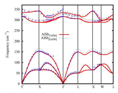
Figure E.2: Transferability of the force constant from GaSb to AlSb. The AlSb band structure has been calculated using the force constant of AlSb (red solid line) and GaSb (black dashed line), and is compared to experimental values reproduced from [99] (blue crosses).
