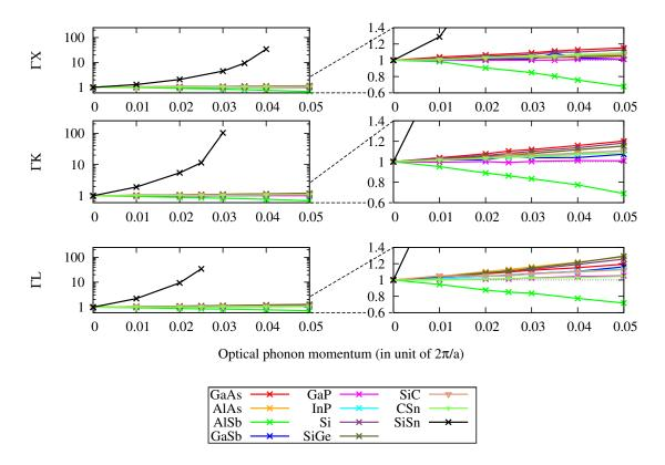
Figure 2.8: Dependence of the bare two-phonon final states number upon the wavevector  $|\mathbf{q}_{LO}|$  of an initial LO-phonon belonging to  $\Gamma X$ ,  $\Gamma K$  and  $\Gamma L$ . For an easier comparison number of final states are normalized to 1 at  $|\mathbf{q}_{LO}| = \mathbf{0}$ .
