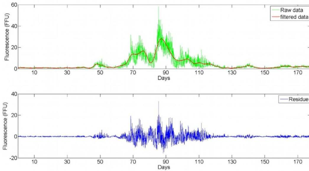
**Figure 13.** Raw fluorescence data for the year 2006, superposed to the trend estimated using the EMD method, modes 12 to 20, corresponding to a smoothing at scale 5 days. Below: the high frequency part, corresponding to the sum of modes from 1 to 11.
