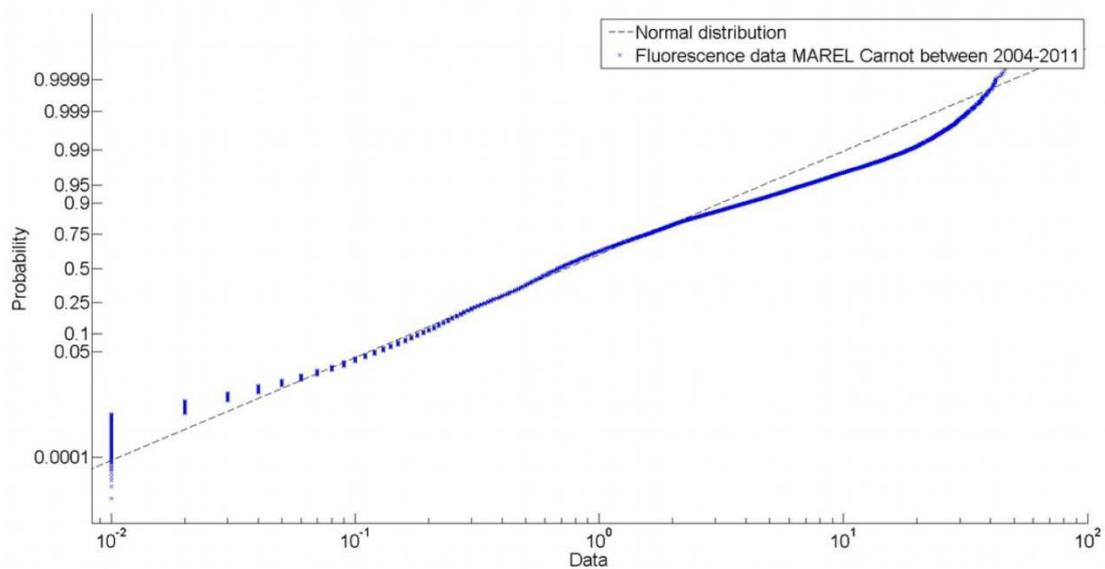
**Figure 5.** Lognormal test of the fluorescence distribution, using the so-called lognormal probability plot; the black line is a straight line corresponding to the lognormal distribution, and the dots are the fluorescence data.
