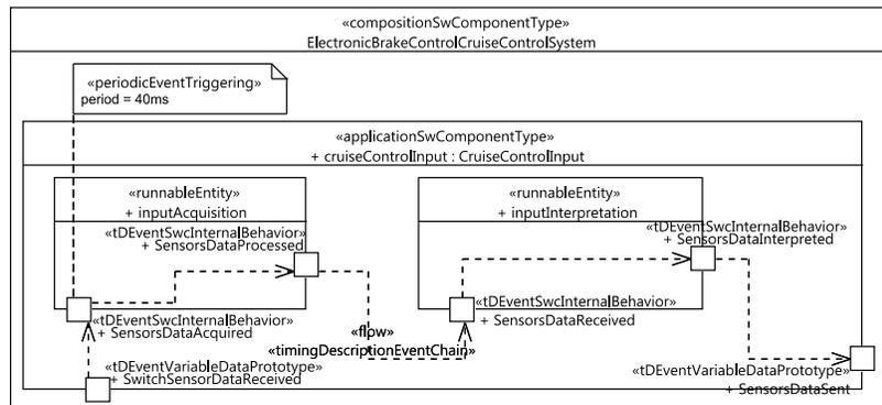
**Figure 5.24. Specification of the Activation Period under the Application Timing Viewpoint (at the AUTOSAR SystemTiming Level)**
