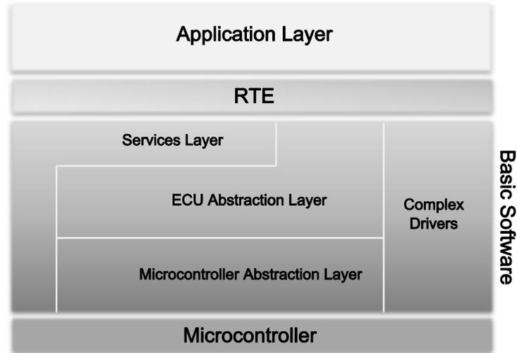
**Figure 2.2. AUTOSAR Architecture Layers Schema**
