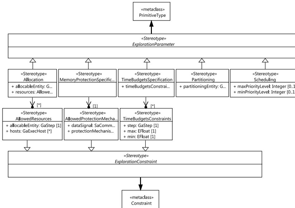
**Figure 5.32. UML Profile for the Exploration Parameters**
