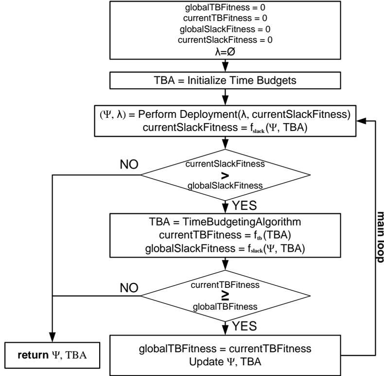
**Figure 4.31. Iterative Improvement Loop for the Staged Approach**
