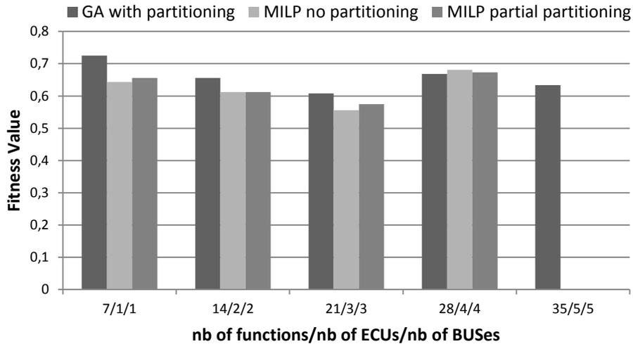
**Figure 4.20. Comparison using Fitness Function ( $0.5 * f_{e2e}(\Psi_i) + 0.5 * f_m(\Psi_i)$ )**
