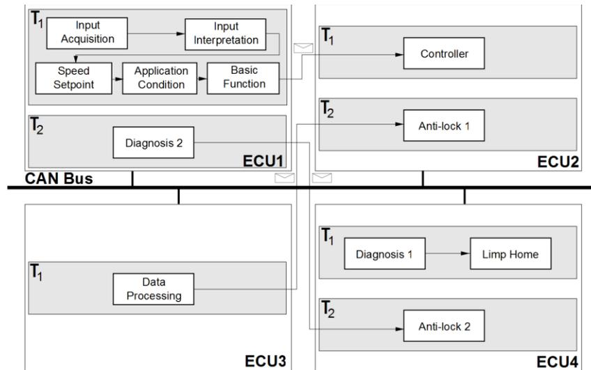
**Figure 4.32. Deployment Configuration for CCS and ABS**
