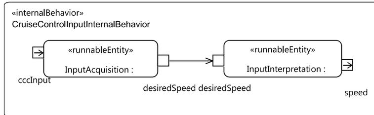
**Figure 5.20. Model of the Internal Behavior for the CruiseControlInput Software Component**
