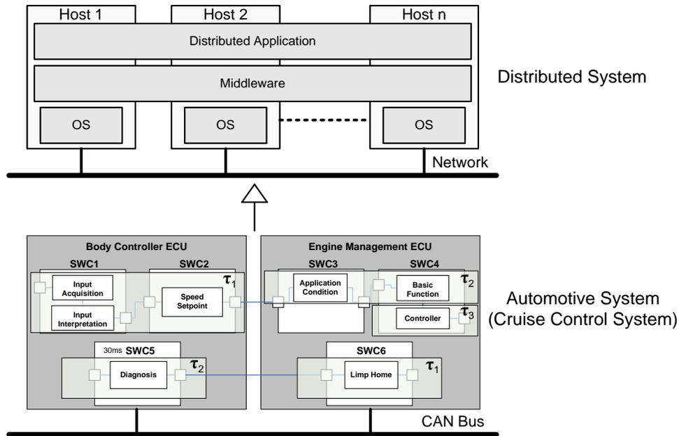
**Figure 1.1. Distributed System and Automotive Distributed System**
