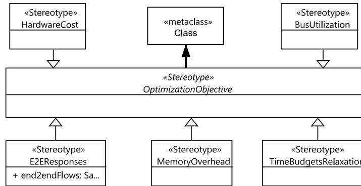
**Figure 5.33. UML Profile for the Optimization Objective**
