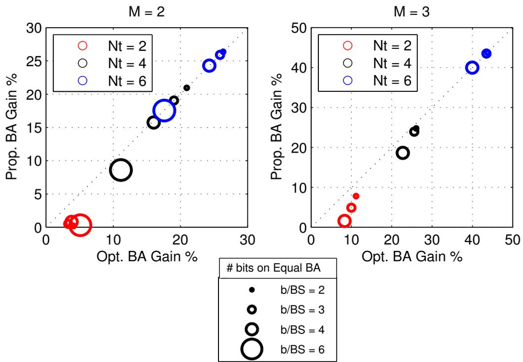
Figure 3.3: Optimal BA vs. Proposed BA gain for CBF at SNR = 0 dB.
