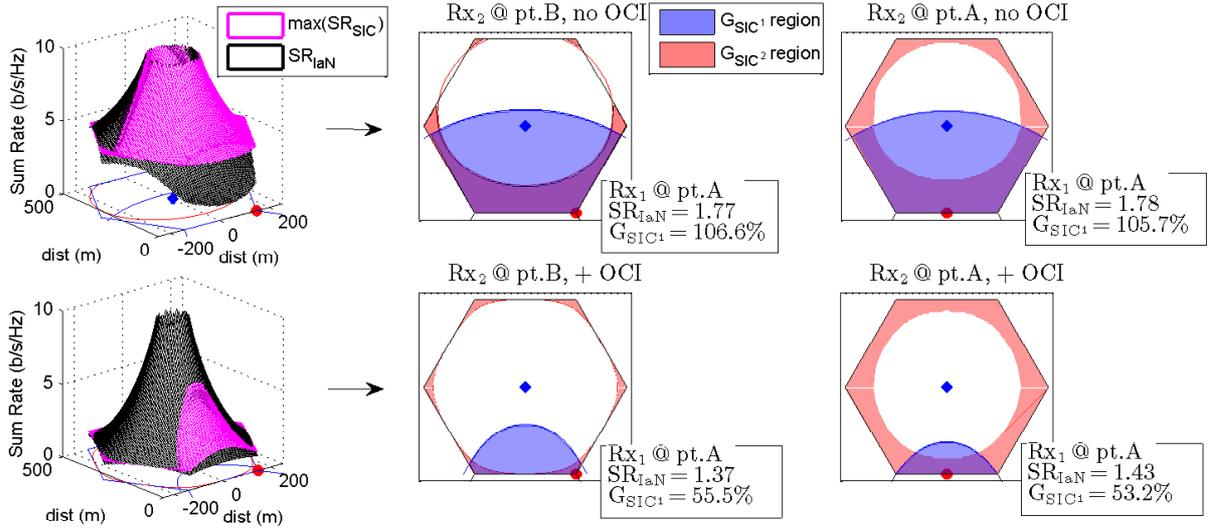
Figure 4.3: Regions for SIC gain conditions. Rx<sub>2</sub> fixed, Rx<sub>1</sub> moves all over cell 1. Minimum received SNR  $p = 5$  dB.
