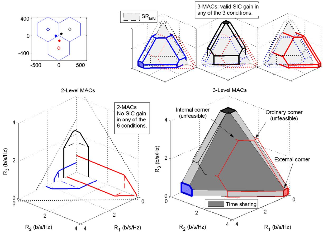
Figure 4.6: MAC levels in a 3 Tx-Rx pairs network.
