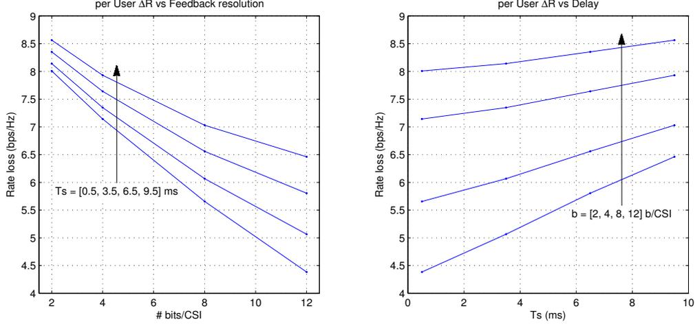
Figure 2.2: Average per user rate offset for CBF with perfect and QD-CSI in the high SNR regime (i.e. SNR = 30 dB) for  $M = 2$ ,  $N_t = 4$ ,  $v = 5$  km/h, and  $f_c = 2.1$  GHz.
