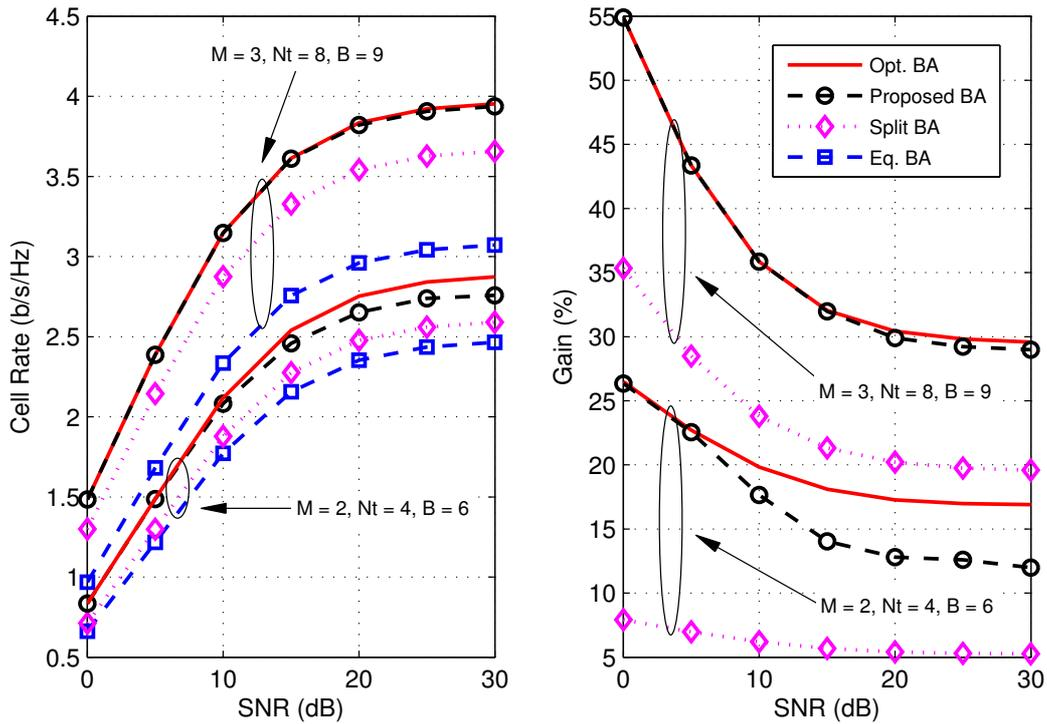
Figure 3.1: Left: Single-cell rates for CBF. Right: Gains with respect to Equal BA.
