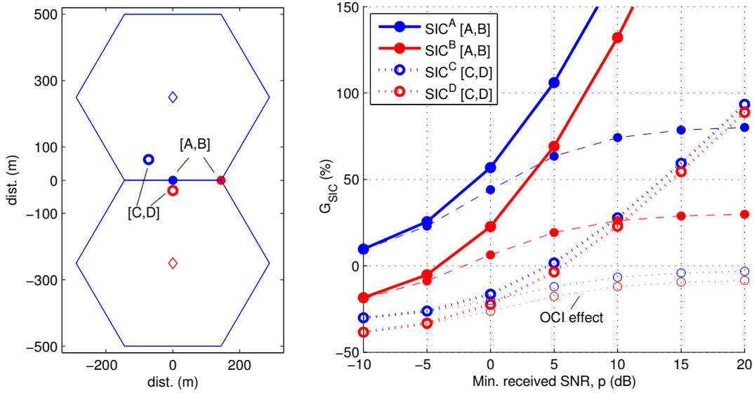
Figure 4.4: SIC gain upper bound and effect of OCI.
