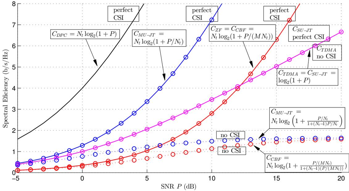
Figure 1.1: Achievable rates for single-cell and multi-cell MISO and MIMO channels.  $N_t = N_r = M = 4$ . Both single-cells and multi-cell schemes use a total system SNR =  $P$  constraint. effective feedback mechanisms which should be designed to improve the TDMA performance ( $d = 1, r = 1$ ), where no cooperation no multiple antennas and no spatial CSI is needed.
