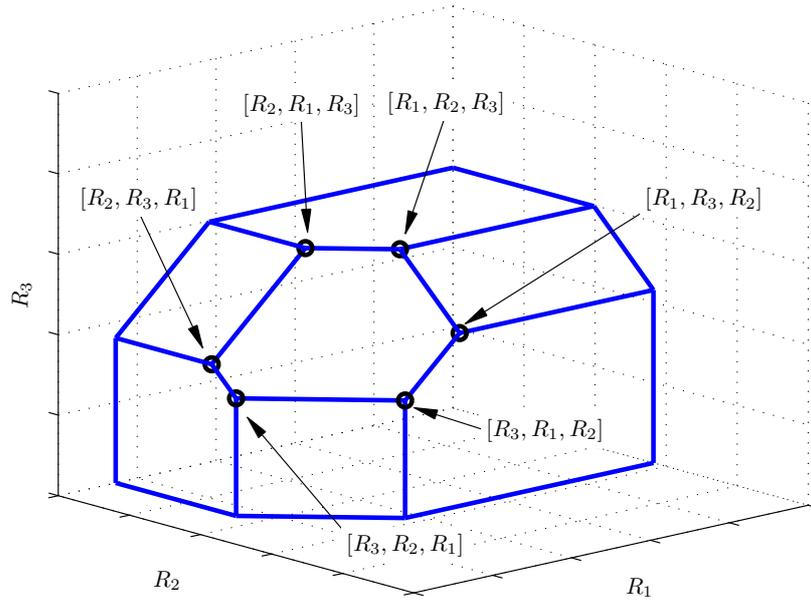
Figure 1.3: Capacity region of the 3-Tx MAC with all possible SIC decoding orders.
