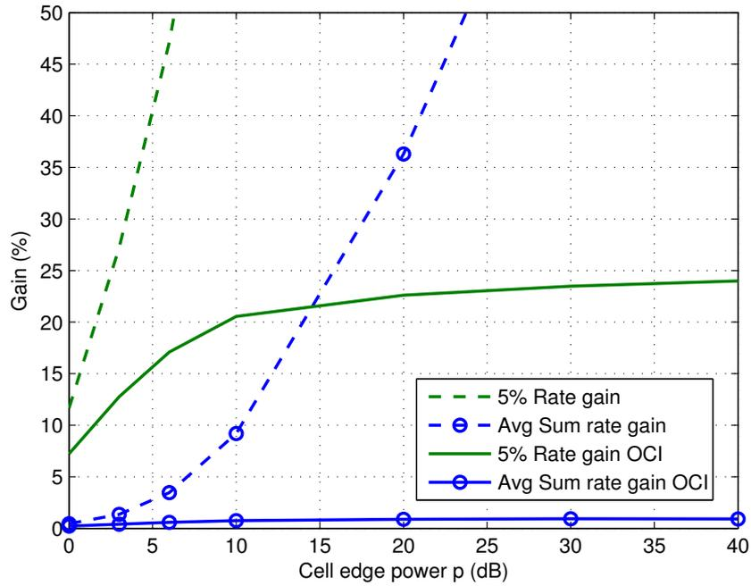
Figure 4.18: Sum rate and 5%-rate gains for radom users in both triangles.
