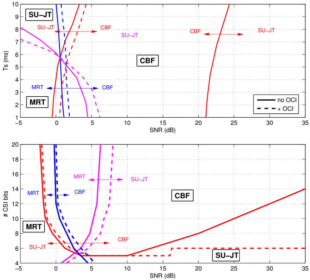
Figure 2.9: Operating regions for different transmit modes with delayed and quantized CSI,  $M = 2$ ,  $N_t = 4$ ,  $v = 10$  km/h. Top: Delay changes with  $b = 8$ . Bottom: Resolution changes with  $T_s = 1$  ms.
