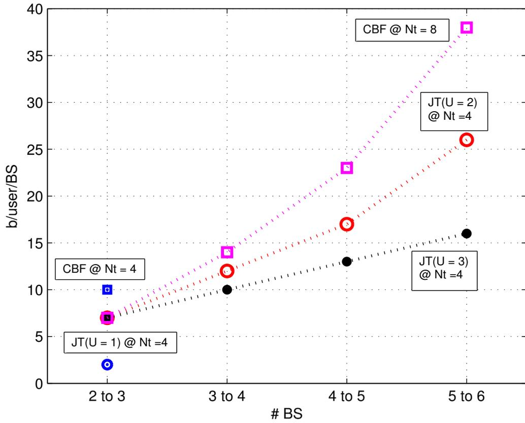
Figure 2.7: Number of CSI bits needed to ensure a sum rate gain of 0.5 bps/Hz, by increasing the number of BS.
