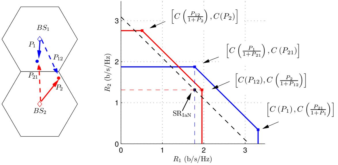
Figure 4.1: A 2x2 IC decomposed in 2 MACs.
