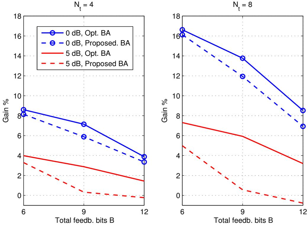
Figure 3.2: Gains w.r.t. Equal BA for JT with  $M = 3$ .
