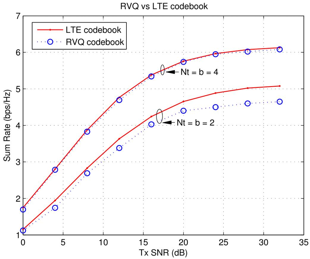
Figure 2.6: Average Sum Rate of CBF systems without OCI for  $M = 2$ ,  $N_t = 4$ , and  $v = 5$  km/h.
