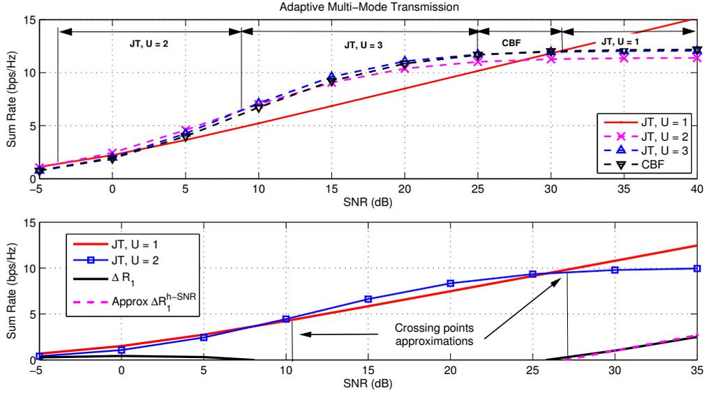
Figure 2.3: Top: Adaptive Multi-mode Transmission for CoMP.  $M = 3$ ,  $N_t = 4$  and  $b = 4$ . Bottom:  $\Delta R$  approximations and crossing points.  $M = 3$ ,  $N_t = 2$  and  $b = 6$ . Both graphs use  $v = 5$  km/h,  $T_s = 1$  ms, and  $f_c = 2.1$  GHz.
