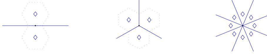
Figure 4.11: The best position for enabling cooperative SIC for 2, 3 or 8 Tx-Rx pairs.
