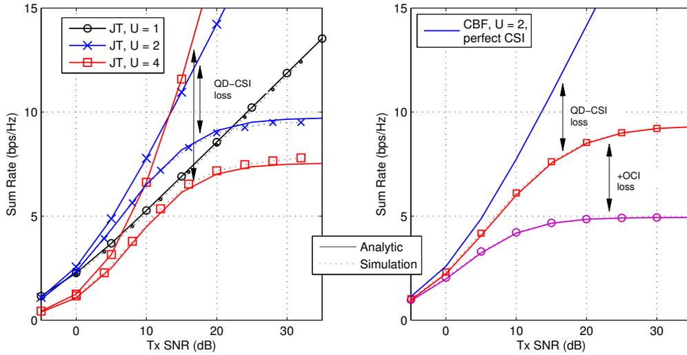
Figure 2.4: Left: Achievable rates for JT with perfect and QD-CSI.  $M = 3$ ,  $Nt = 4$ ,  $b = 10$ , and  $v = 10$  km/h. Right: Achievable rates for CBF including perfect CSI, QD-CSI and the effect of OCI.  $M = 2$ ,  $Nt = 4$ ,  $b = 8$ , and  $v = 5$  km/h.
