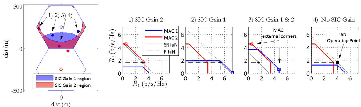
Figure 4.2: SIC Gain regions: user 2 is fixed and user 1 is placed in four different positions.
