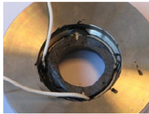
Figure 43. Electrical test conducted on cup-shape ceramic disk
