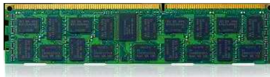
Figure 2.3: An advanced Samsung DDR3 DRAM module [9].
