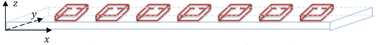
Figure 3. 4: non-located piezoelectric patches bonded on a beam of the same width
