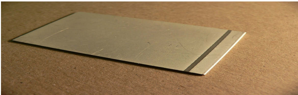
Figure 6.1 : Wrap around electrode (WAE) piezoelectric patch provided by Noliac, Inc
