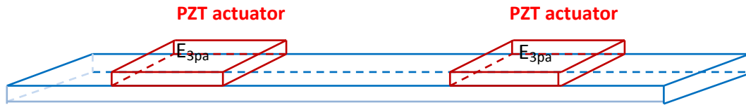
Figure 7.15: System 2: two modes excitation
