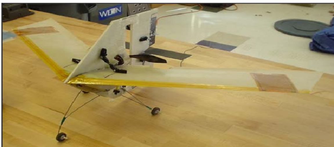
Fabricated micro air vehicle using MFC actuator [ (Bilgen, 2007)]
