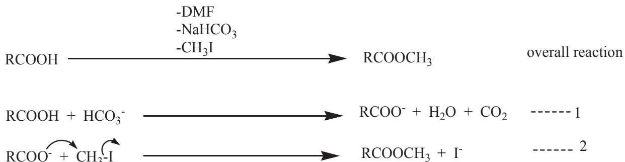
Scheme 13. Reaction mechanism of methylation of carboxylic acid
