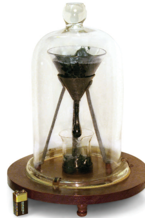
(b) Pitch Drop Experiment. (Credit: John Mainstone, University of Queensland under Creative Commons)
