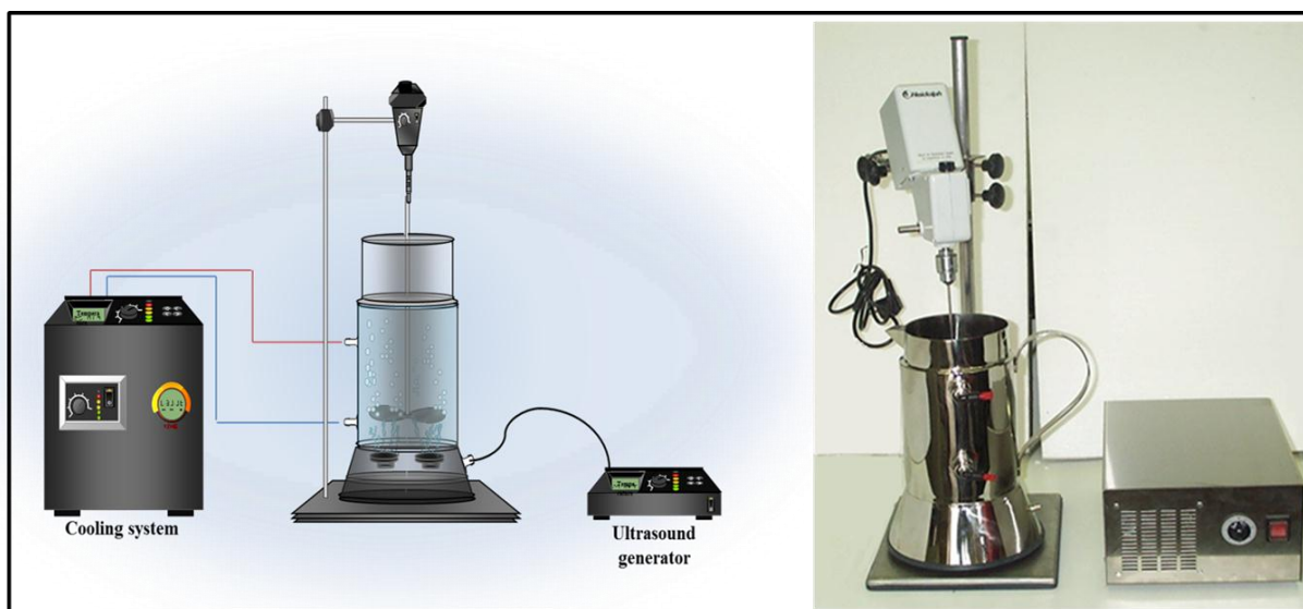
Figure I.9. Ultrasound apparatus used for extraction procedures (scheme and picture).
