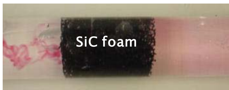
Figure 1-10. (A) Optical photo of the medium to high specific surface area (from 10 to 100 m 2 ·g -1 ) porous silicon carbide support with different macroscopic shapes ranged from 10 -6 m to 10 -1 m. (B) Flow mixing through a SiC foam which acting as a static mixer. Courtesy by SICAT SARL. [136]
