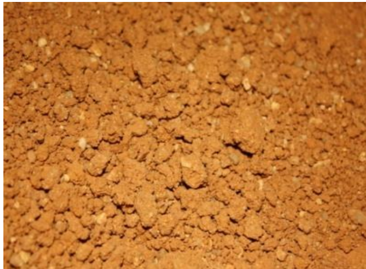
Figure III.1. Sable de Missillac
