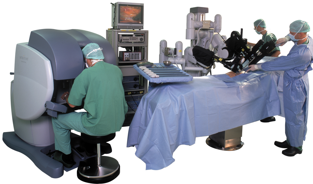
Fig. 3.3. First generation of the da Vinci surgical system by Intuitive Surgical (©2013 Intuitive Surgical, Inc.).
