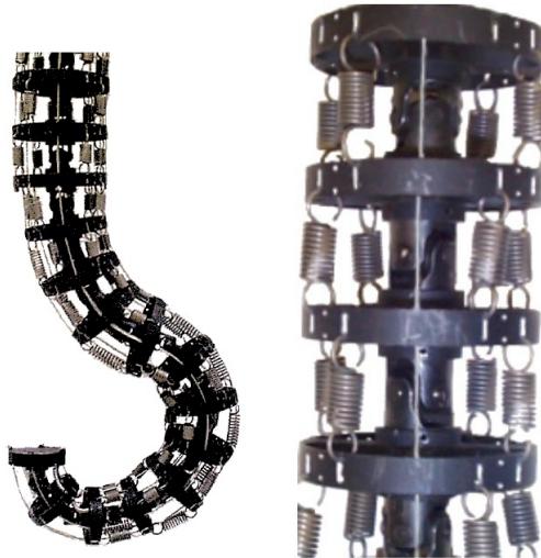
Fig. 4.5. Elephant Trunk manipulator by Clemson University. Left: global view. Right: detail of a section (reprinted from [70]).
