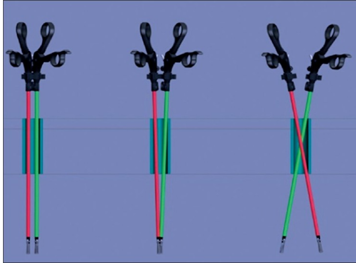
Fig. 2.23. When instruments are inserted from a narrow port, they enter almost parallel inside the body, and their triangulation is compromised. If the trocar is large enough to deviate their path, then the problem becomes the instruments inversion: the instrument that appears on the left in the image is controlled by the right handle and vice versa (reprinted from [40]).
