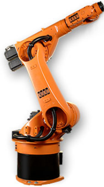
Fig. 4.1. The Kuka KR 30-3, an anthropomorphic manipulator for medium payloads (courtesy of Kuka Roboter GmbH, Augsburg, Germany).
