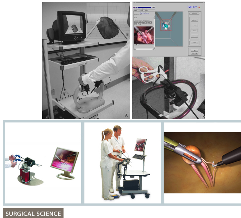
Fig. 5.5. Top: The MIST-VR simulator by Mentice AB (reprinted from [95], [159]). Bottom: LapSim simulator by Surgical Science Sweden AB (reproduction from http://www.surgical-science.com ).
