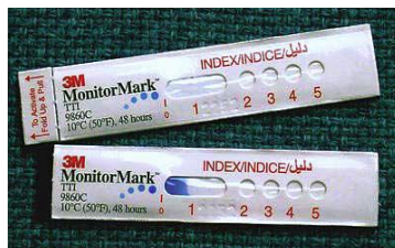
Figure 1-I.10. 3M™ MonitorMark™ labels - The blue dye continues to diffuse while the melting point is exceeded
