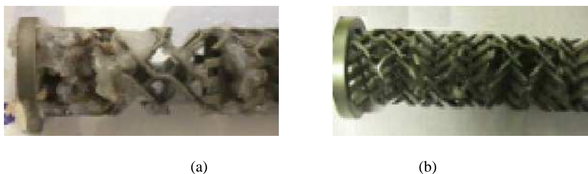
Figure 2.16. Fouled static mixer due to precipitation of high molecular weight acrylic polymer (a), clean static mixer after premixing of the reactant by a micromixer (b). 97
