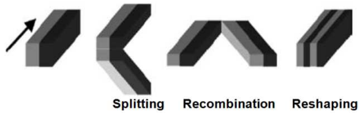
Figure 2.19. Schematic of split and recombine principle. 99
