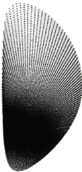
Figure 2.2: Initial polar grid for Bézier elements (poloidal plane) in the ITER case (standard H-mode scenario 15MA/5.3T , described in section 3.4).
