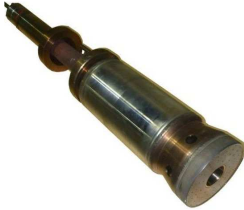
Figure 1.6: Multi-volume damper based on coupled Helmholtz resonating cavities [Bothien et al. (2013)]. Courtesy of Dr. M. Bothien.
