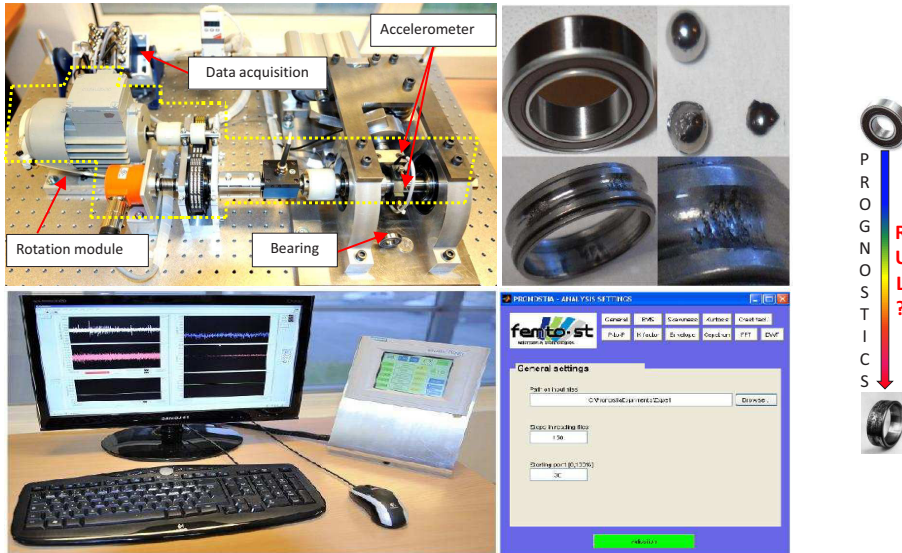
FIGURE 2.8: PRONOSTIA testbed - FEMTO-ST Institute, AS2M department
