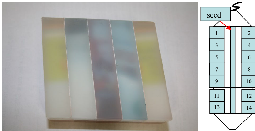
Fig.5.2: Quartz crystal bars and their positions in the crystal.
