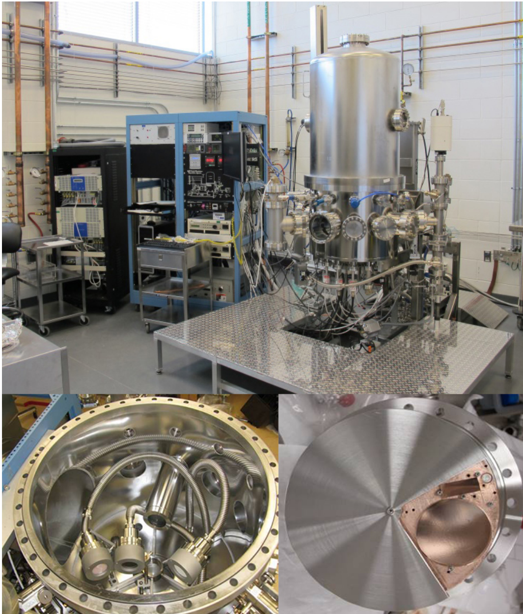
Figure V.1.6: The UHV deposition system (top) , setup inside the chamber(bottom left) and sample holder (bottom right)
