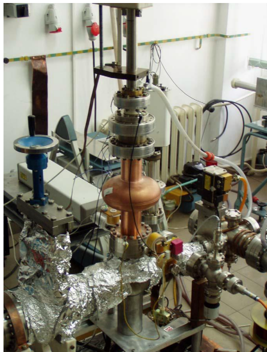
Figure I.3.5: Arc deposition system for the ARCO project [99].
