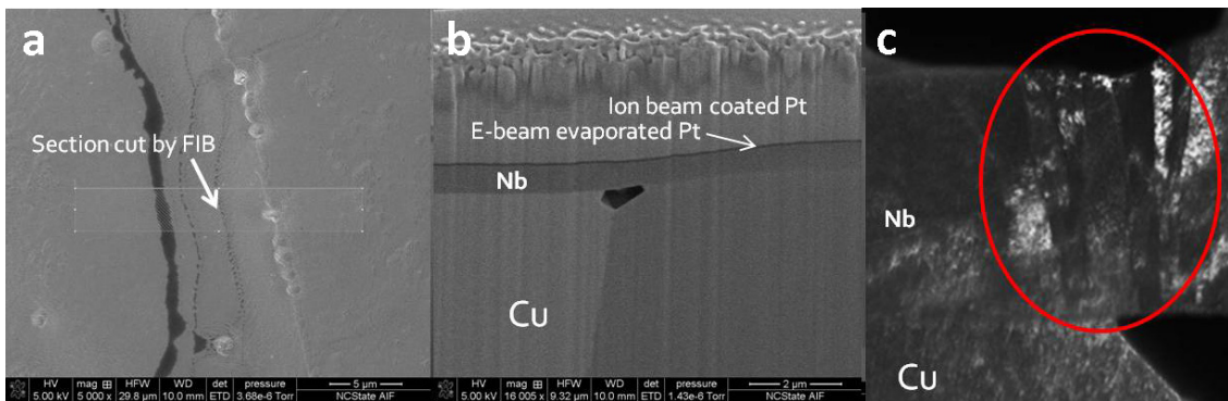
Figure IV.2.25: (a), SEM micrograph of an ECR Nb/Cu film at the location of FIB cut (b) FIB cross section revealing a void in the Cu substrate near the surface, (c) TEM cross section in dark field revealing the resulting ab-normal growth in the Nb film.
