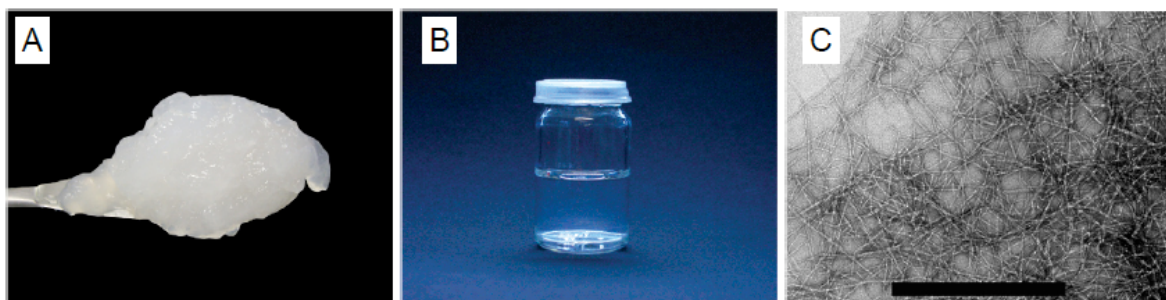
Figure 36. Microfibrillated cellulose. (A) Wood pulp recovered after high pressure homogenization of wood. 146 (B) Solution of MFC (1.9 g/L) obtained after dilution of the pulp, ultrasonication and centrifugation. (C) TEM images of the MFC from solution described in (B). The scale bar is 500 nm. 148
