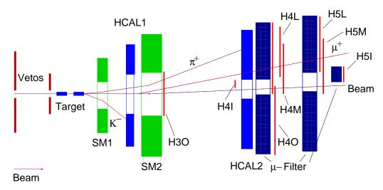
Figure 2.13: Schematic view of the trigger system. The most upstream veto and the H1G and H2G hodoscopes are not shown.
