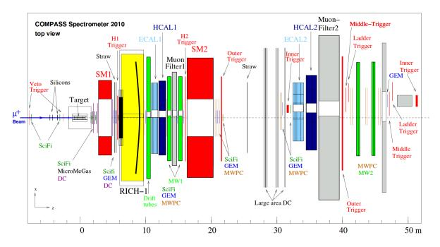
Figure 2.8: Sketch of the top view of the COMPASS muon setup (as built in 2010, no change compared to 2011).
