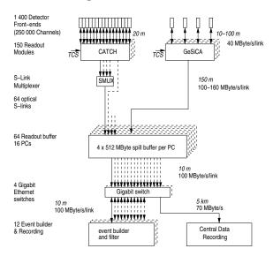
Figure 2.16: General structure of the DAQ system. It mainly consists on three stages: digital signals collection, the readout modules, partial events storage, the readout buffer PCs, and event records, the event builder (see text).
