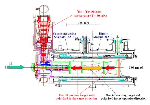
Figure 2.7: Sketch of refrigerated polarised target. The arrows indicate the orientation of the polarisation for each target cell. The geometrical acceptance of the target is limited to  $\pm 180$  mrad defined by the radius of the solenoid.
