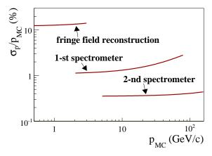
Figure 2.9: Relative track momentum resolution  $\sigma_p/p$  versus p.
