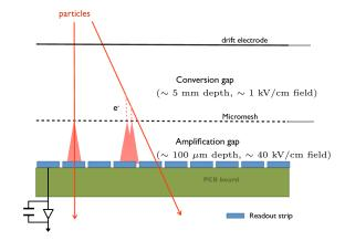
Figure 2.10: Principle of a Micromegas detector.
