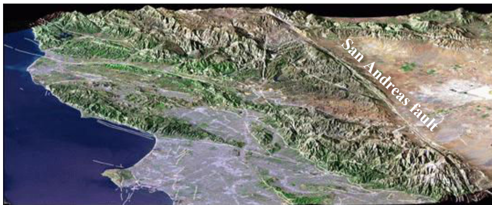
Fig. 13 : Landsat and topographic map view of the San Andreas Fault system (white lines) made of the major San Andreas strike-slip fault and of an associated dense network of smaller strike-slip and reverse faults (from http://earthobservatory.nasa.gov/IOTD/view.php?id=3067 )
