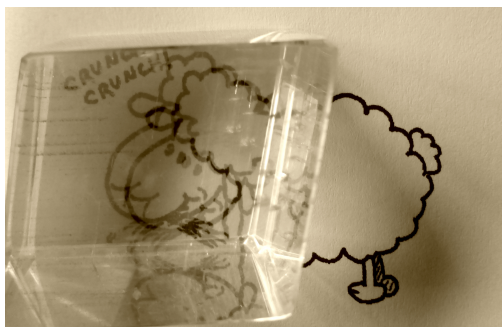
FIGURE 1.1: An example of birefringence: the drawing of the sheep is split into two parts when looked through the birefringent crystal.
