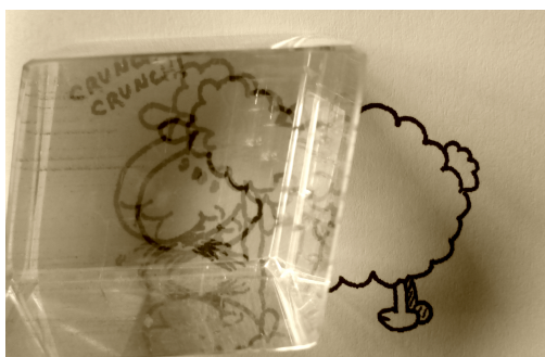
FIGURE 1.1: An example of birefringence: the drawing of the sheep is split into two parts when looked through the birefringent crystal.
