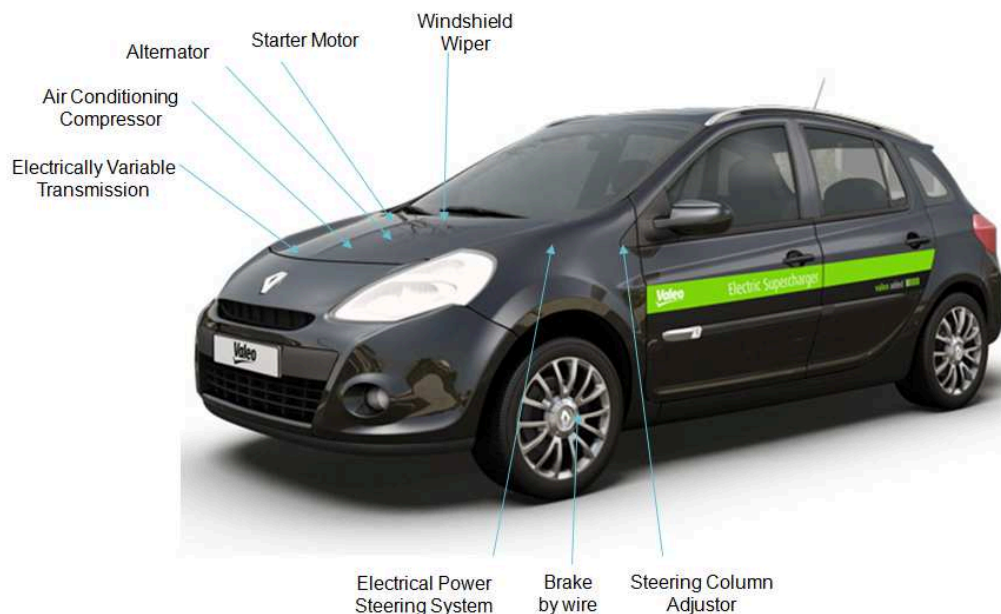
Figure 1.1 Electrical Drives in Vehicle [courtesy of Valeo]
