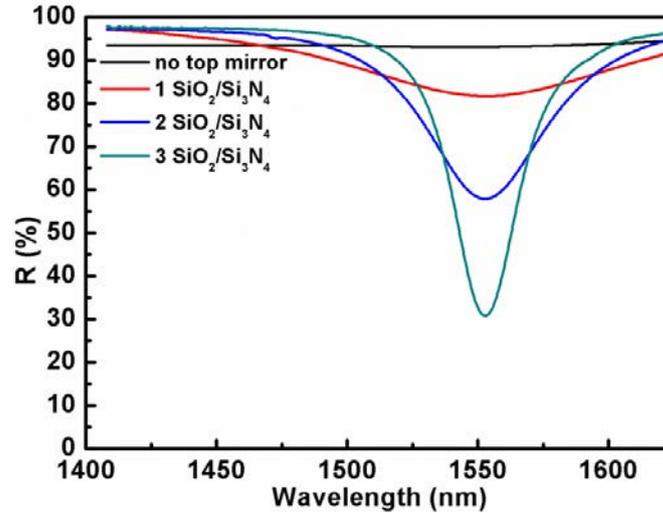
Figure 4.18: The linear reflectivity spectra of the GSAMs with the top mirrors of 0, 1, 2, 3 SiO<sub>2</sub>/Si<sub>3</sub>N<sub>4</sub> layer pairs, respectively.
