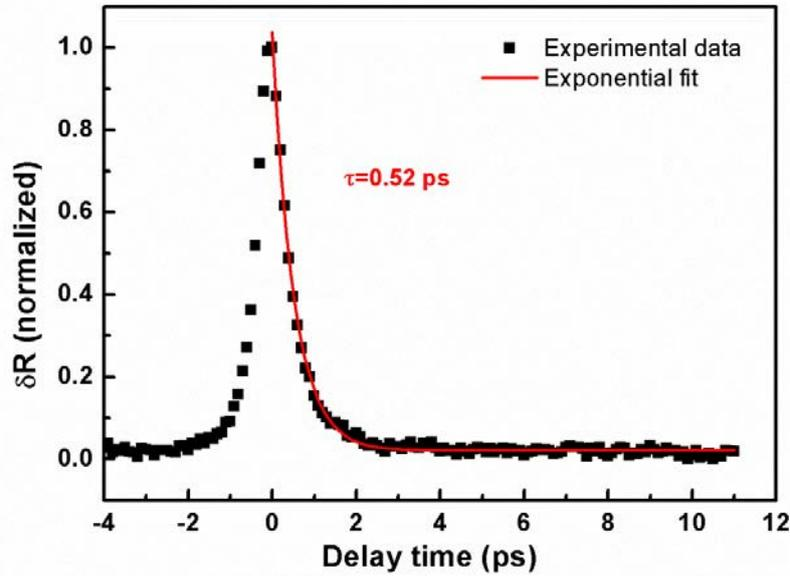
Figure 2.14: Normalized transient reflection as a function of the pump-probe delay for the As<sup>+</sup> implanted sample with the ion dose of  $1.3 \times 10^{12}$  ions / cm<sup>2</sup> without annealing.
