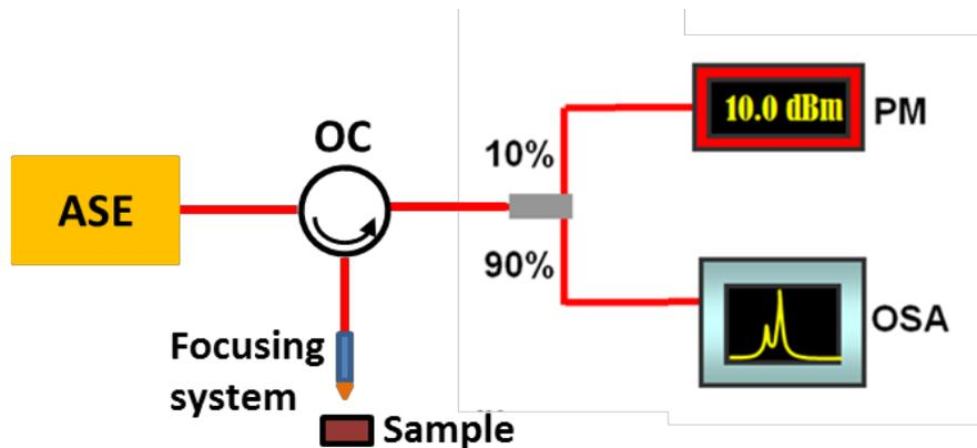
Figure 3.19: Experimental setup for measuring linear reflection spectrum.
