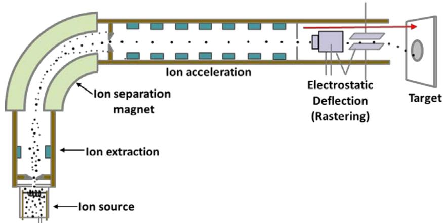
Figure 2.5: Schematic overview of an ion implanter.
