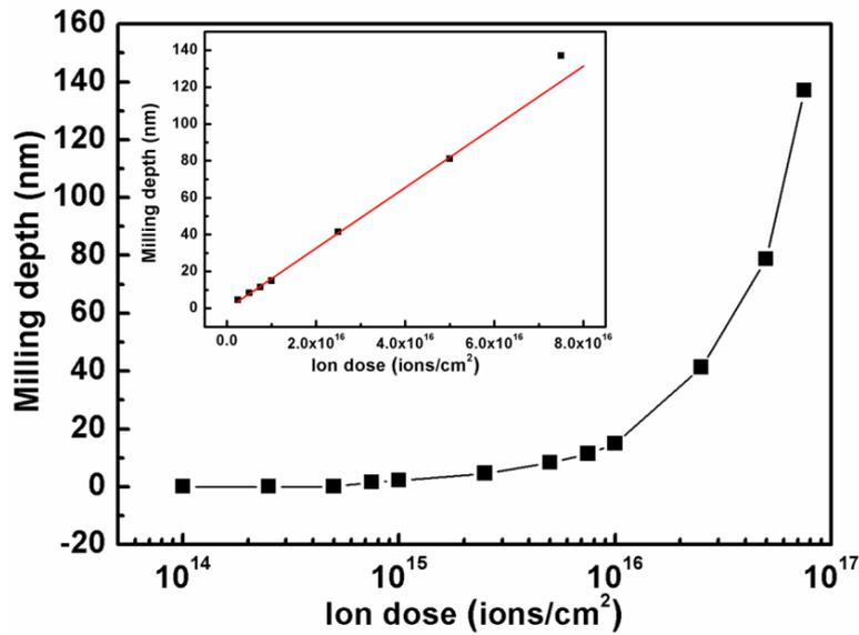
Figure 3.15: Average milling depths as a function of incident ion dose from  $1 \times 10^{14}$  to  $7.5 \times 10^{16}$  ions/cm<sup>2</sup>, in semi-logarithmic scale. The inset is the relationship between average milling depth and ion dose from  $2.5 \times 10^{14}$  to  $7.5 \times 10^{16}$  ions/cm<sup>2</sup>, in linear scale.
