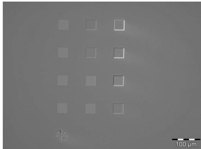
Figure 3.13: Optical microscopy image (top view) of 3×4 FIB-patterned square array with the ion doses ranging from  $1 \times 10^{14}$  ions /  $\text{cm}^2$  (bottom left-mark#1) to  $7.5 \times 10^{16}$  ions /  $\text{cm}^2$  (top right-mark#12). The size for each square is  $35 \times 35 \mu\text{m}^2$ .
