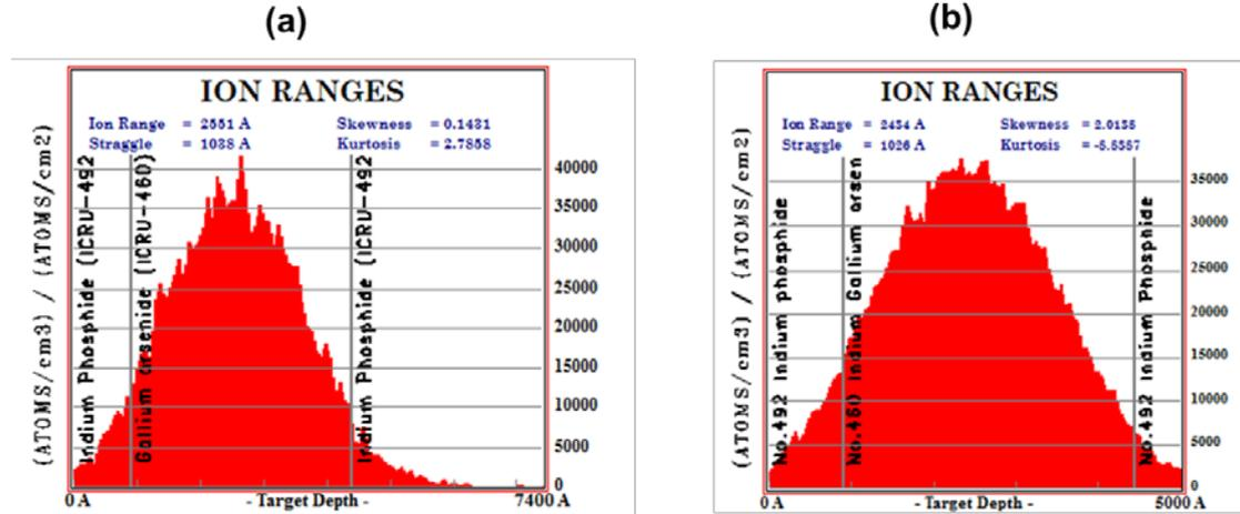
Figure 2.10: TRIM simulation: (a) As atoms distribution in the InGaAs active region, (b) Fe atoms distribution in the InGaAs active region.
