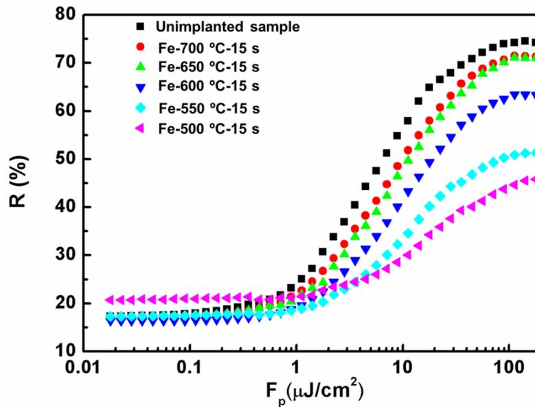
Figure 2.20: Reflectivity of the unimplanted sample and the Fe<sup>+</sup>-implanted samples after annealing at 500 °C, 550 °C, 600 °C, 650 °C, 700 °C for 15 s as a function of the input energy fluence.
