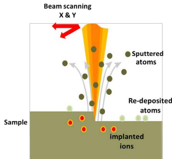
Figure 3.9: Schematic representation of the FIB milling process.
