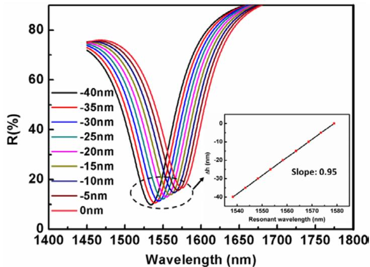
Figure 3.3: Resonant wavelengths as a function of change in the thickness of the top phase layer.
