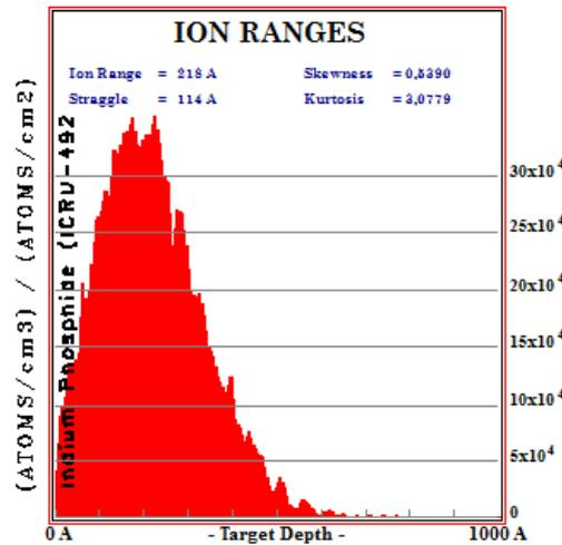
Figure 3.10: TRIM simulation plots of 30 keV  $\text{Ga}^+$  into InP: depth distribution of Ga ion.
