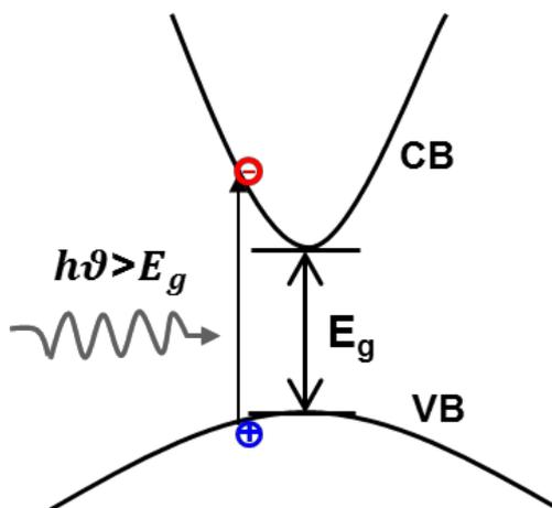
Figure 2.2: Optical absorption in a direct band-gap semiconductor.
