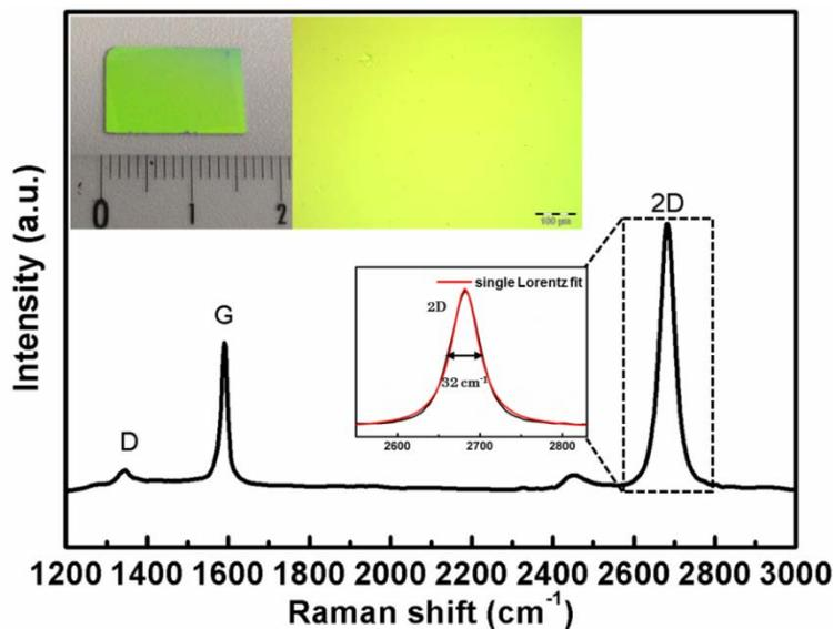
Figure 4.15: Raman spectrum of the SLG on bottom mirror with a 532 nm excitation laser (The Raman signal of bottom mirror was subtracted). The 2D peak was fitted with a single Lorentz peak. The insets are the photo and the microscope image of the SLG on bottom mirror, respectively.
