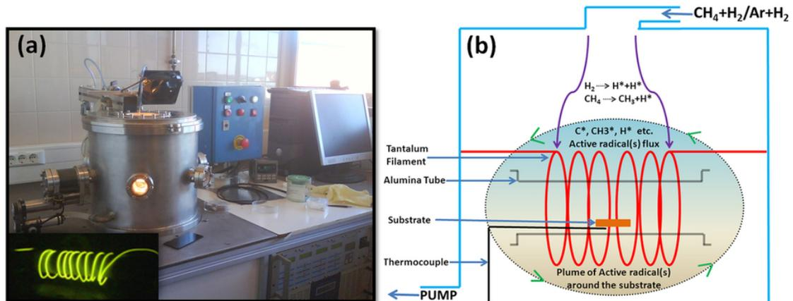
Figure.4.13: (a) Homemade (LPN-CNRS) hot filament thermal CVD set-up for large-area graphene film deposition. Inset shows Ta filament ( $\sim 1800$  °C) wound around alumina tube. (b) Schematics of graphene growth deposition and formation of active flux of highly charged carbon and hydrogen radicals by catalytic reaction of gaseous precursors with the filament.
