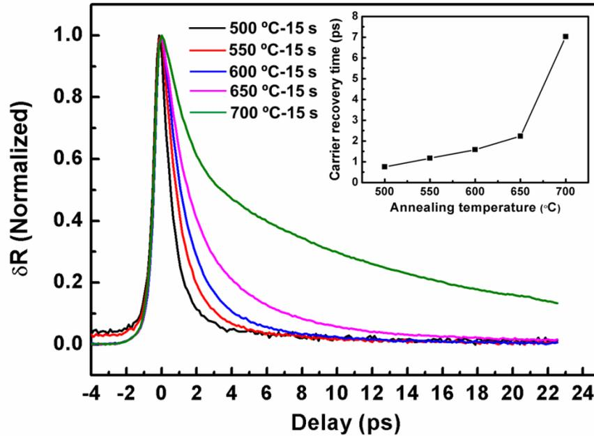
Figure 2.17: Normalized transient reflection as a function of the pump-probe delay for the Fe<sup>+</sup> implanted samples with the dose of  $1 \times 10^{14}$  ions / cm<sup>2</sup> after annealing at 500 °C, 550 °C, 600 °C, 650 °C, and 700 °C for 15 s. The inset is the carrier recovery time as a function of the annealing temperature.
