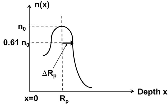
Figure 2.7: Gaussian distribution of the stopped atoms.
