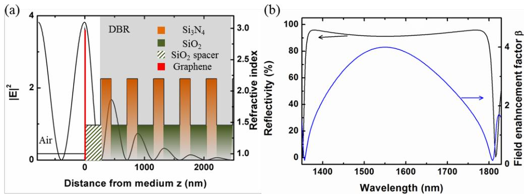
Figure 4.9: (a) Optical field distribution of a GSAM. SiO<sub>2</sub> is in green, Si<sub>3</sub>N<sub>4</sub> is in orange, while the green patterned region is the SiO<sub>2</sub> spacer and graphene is in red on top; the material refractive index profile is in color, and the normalized field intensity  $|E|^2$  is plotted (black curve). (b) Linear reflectivity (black) and field enhancement factor (blue) of the GSAM as a function of the wavelength.
