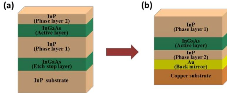
Figure 3.16: (a) As-grown structure, (b) Microcavity-based structure.
