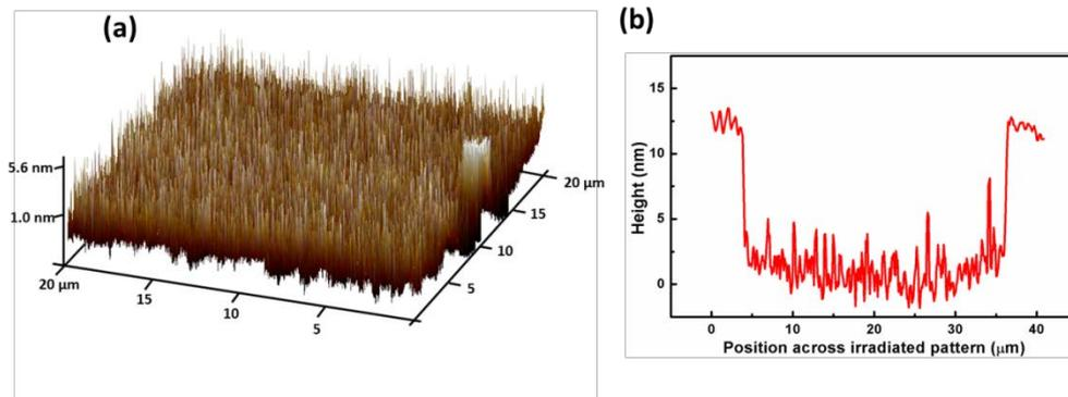
Figure 3.14: AFM characterizations on an irradiated zone of InP substrate. The dose is  $5 \times 10^{15}$  ions /  $\text{cm}^2$ . (a) Surface roughness measurement of the milled area. The scan size is  $20 \times 20 \mu\text{m}^2$ , RMS is 1.18 nm. (b) A typical cross section of the surface profile, as obtained from the AFM scan.
