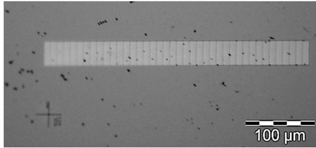
Figure 3.17: Optical microscopy image (top view) of the taper structure fabricated with the ion doses ranging from  $1.5 \times 10^{16}$  ions /  $\text{cm}^2$  (left-mark#1) to  $2.5 \times 10^{16}$  ions /  $\text{cm}^2$  (right-mark#40). The size for each rectangle is  $35 \times 10 \mu\text{m}^2$ .
