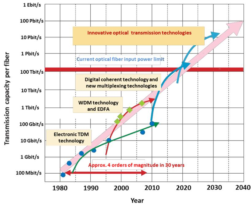
Figure 1.1: Evolution in fiber-optic communication technology (commercial trend)
