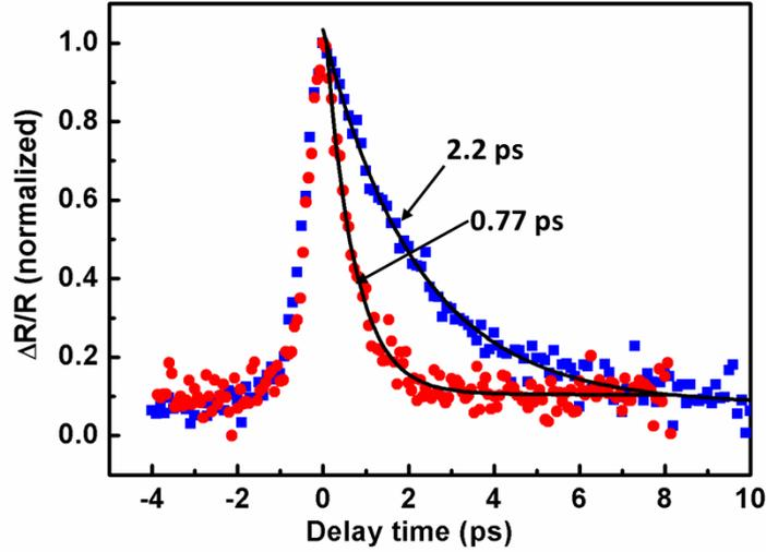
Figure 4.17: Normalized differential reflection changes as a function of pump-probe delay and exponential fit curves for the SLG sample before and after  $\text{Si}_3\text{N}_4$  protective layer deposition.
