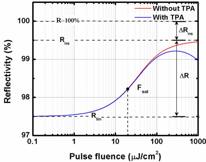
Figure 2.18: Nonlinear reflectivity  $R$  of a SESAM as a function of the logarithmic scale of the incident pulse energy fluence  $F_p$ .  $R_{lin}$ : linear reflectivity;  $R_{ns}$ : reflectivity with saturated absorption;  $\Delta R$ : modulation depth;  $\Delta R_{ns}$ : nonsaturable losses in reflectivity;  $F_{sat}$ : saturation fluence. The red curves show the fit functions without TPA absorption ( $F_p \rightarrow \infty$ ) while blue curves including TPA absorption.
