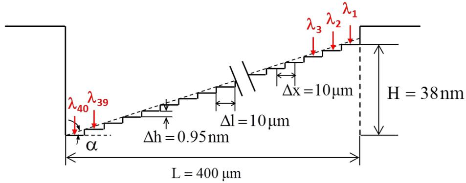
Figure 3.6: Schematic drawing of a taper structure (cross section view).
