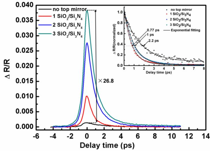
Figure 4.19 Differential reflection changes as a function of pump-probe delay for the GSAMs with the top mirrors of 0, 1, 2, 3  $\text{SiO}_2/\text{Si}_3\text{N}_4$  layer pairs, respectively. Inset is the normalized differential reflection changes as a function of pump-probe delay.
