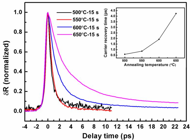
Figure 2.16: Normalized transient reflection as a function of the pump-probe delay for the  $\text{As}^+$  implanted samples with the ion dose of  $1 \times 10^{14}$  ions /  $\text{cm}^2$  after annealing at 500 °C, 550 °C, 600 °C, and 650 °C for 15 s. The inset is the carrier recovery time as a function of the annealing temperature.
