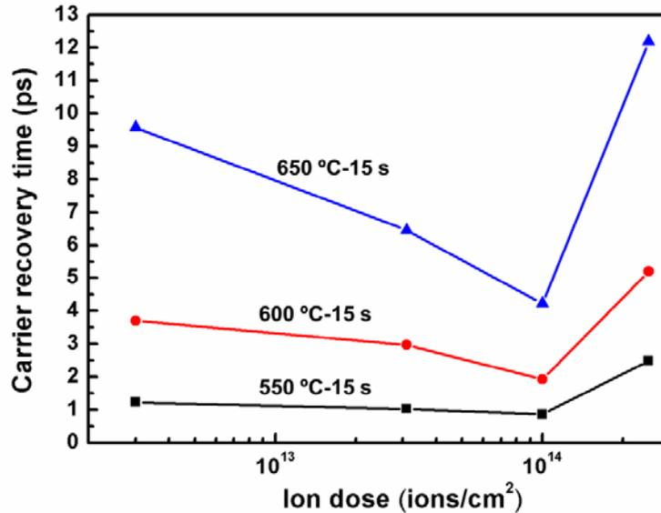
Figure 2.15: Variation of the carrier recovery times versus Arsenic ion dose after rapid thermal annealing at  $550 \text{ }^\circ\text{C}$ ,  $600 \text{ }^\circ\text{C}$ , and  $650 \text{ }^\circ\text{C}$  for 15 s.
