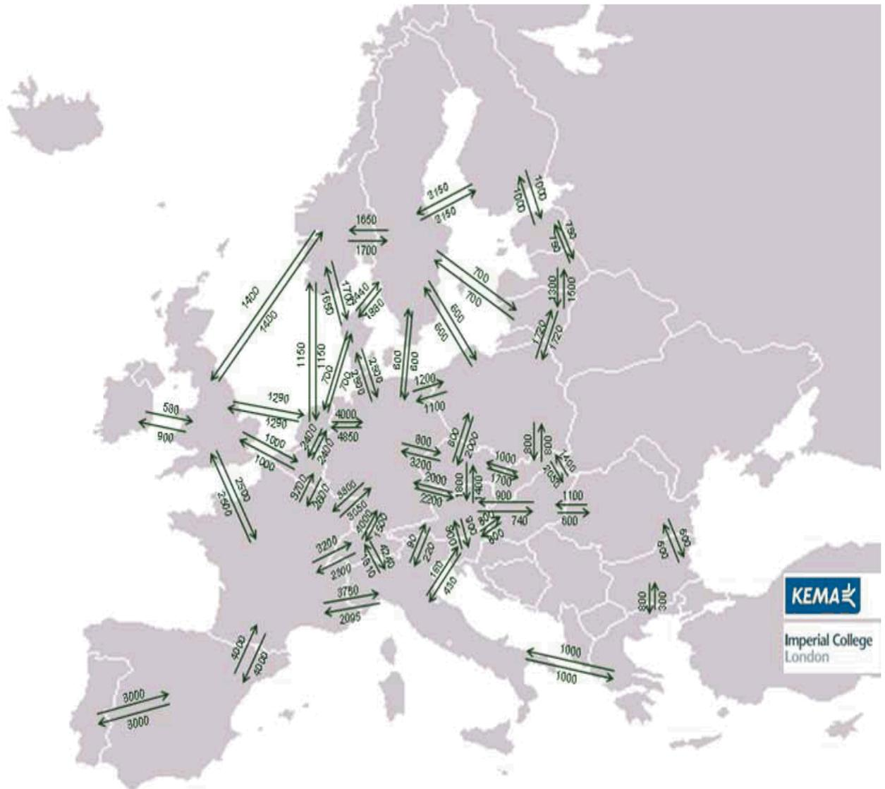
**FIGURE 7.1 SCHEMA D'INTERCONNEXION EUROPEEN ANTICIPEE EN VUE DE L'INTEGRATION D'ENR (EN MW)**
